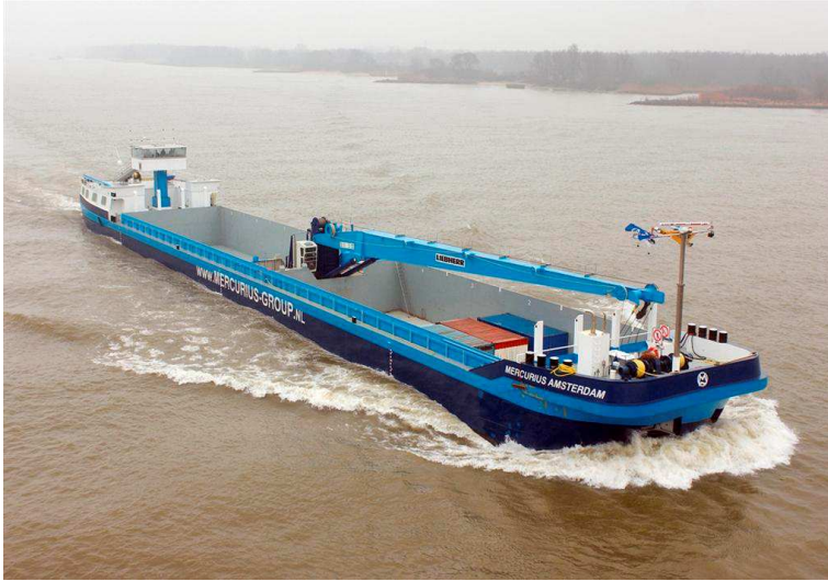
Figure 6.9 A self(un)loading container vessel in The Netherlands
