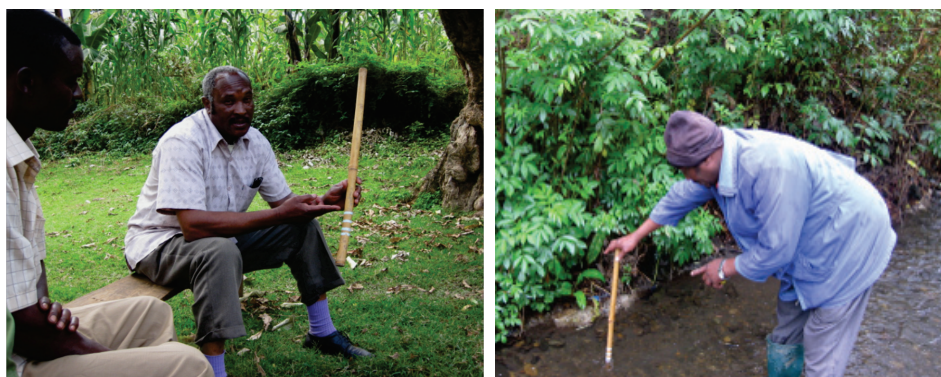
Figure 7.4. The Ngarenaro RC chairman explains the marking of the measurement stick and demonstrates how it is used.
