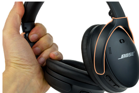
Figure 87: The U-shaped yoke connection in headphones
