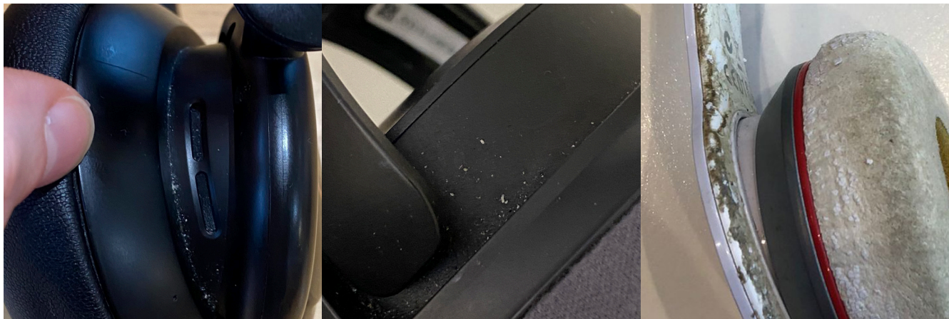
Figure 30: Accumulated dirt in the connection points between the cup and the headband
