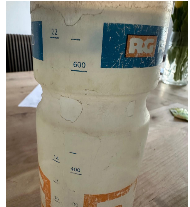
Figure 8: Plastic water bottle with mould on inside and scratches and flaking plastic on the outside
