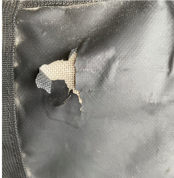
Figure 19: Crackling and peeling polyester plastic of a backpack (Author's image)
