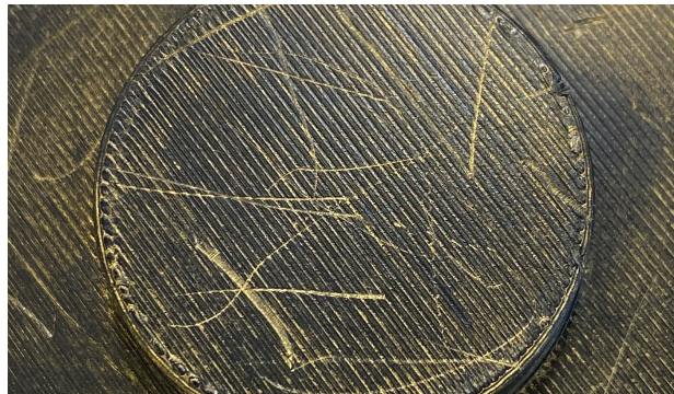
Figure 64: Printing lines showing and plastic turning grey after sanding
