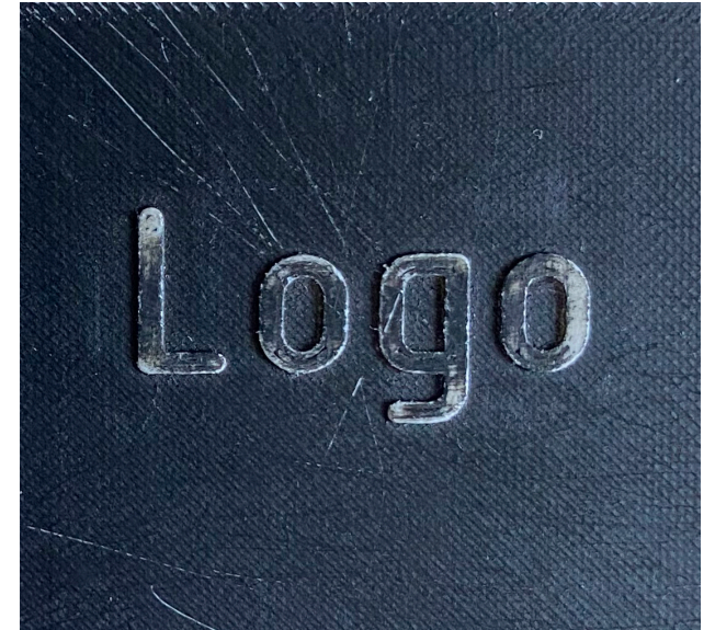
Figure 80: Abrasion test result on the sample with embossing and two layers of solvent-borne paint
