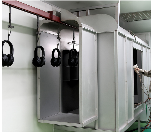
Figure 84: The process of spraying the headphones black with a solvent-borne coating.
