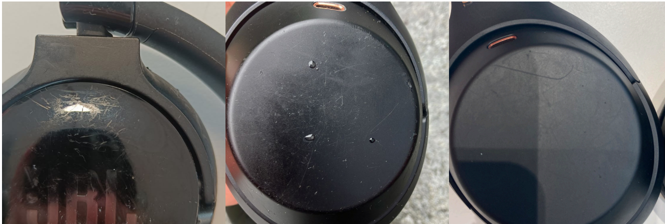
Figure 29: Abrasion in cups with glossy, semi-gloss, and matt finishes
