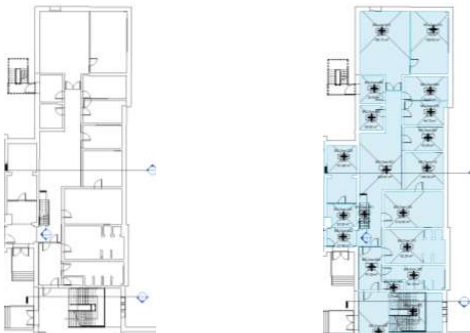
Figure 7: The difference between the physical and the enriched BIM/IFC model
