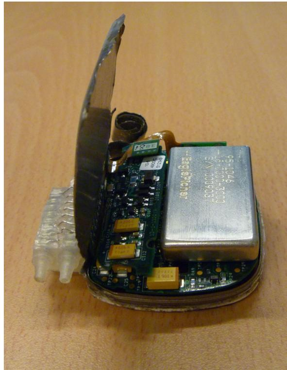
**Figure 1-3:** Picture of an IPG cut open. The battery consumes roughly half the total volume
