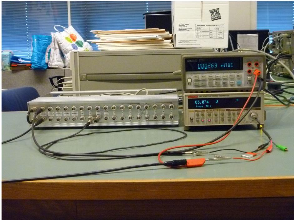
**Figure 7-7:** Source unit and measurement equipment used for testing the prototype
