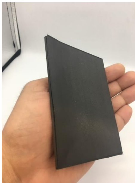
Figure 46 - Poor interlayer adhesion seen in QI specimens (trial specimen)
