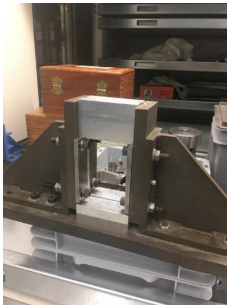
Figure 33 - Fixture used for compression tests of laminates
