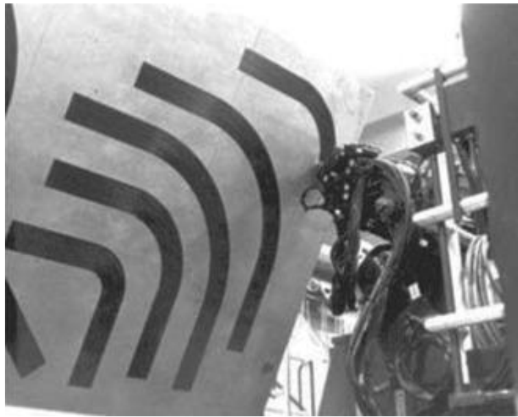
Figure 4 – Fibre tows being steered during deposition using AFP process [8]
