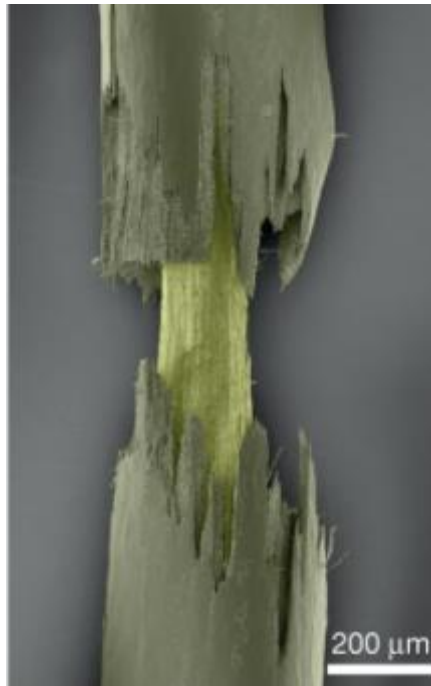
Figure 54 - SEM image of tensile-tested filament specimen [70]
