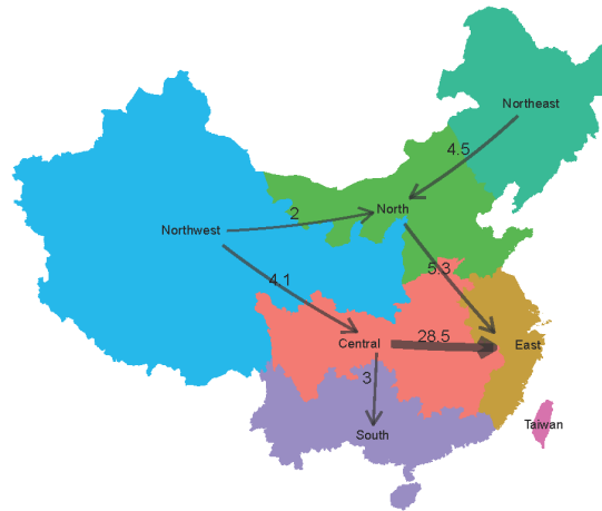
Figure 2.12 – The capacity of the inter-regional transmission network by 2012 in GW. This capacity data is mainly achieved from (Chen et al., 2014) with adaptations for integrating Tibet into the Northwest regional power system.
