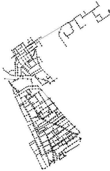
Figure 3.7: Full sewer network of Delft as it is used in all simulations.
