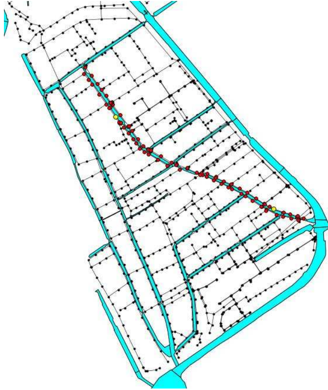
Figure 4.1: Network used for the calibration of surface areas in the simple case. The red nodes are the ones where the surfaces are actually calibrated. The two yellow nodes are the locations used in the visualization of waterlevels in time.
