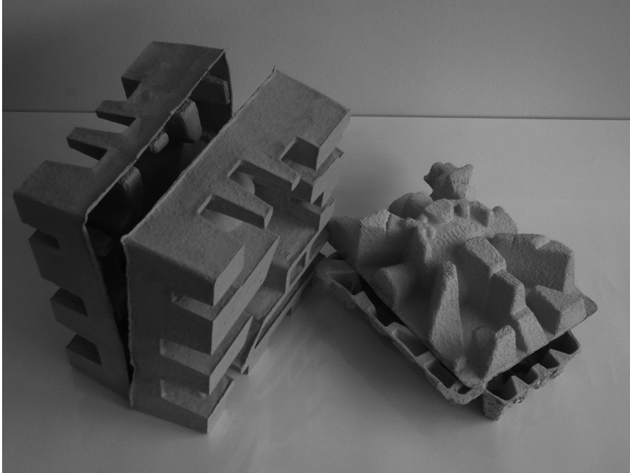
Figure 7.3: Design variety within a particular cushioning solution. The cushioning of two subsequent generations of the Philips Senseo coffee maker. On the left the first generation, which consisted of side cushions, on the right the second generation, which consisted of top and bottom cushions. Both are molded fiber cushions. The resulting outer box dimensions were nearly identical.
