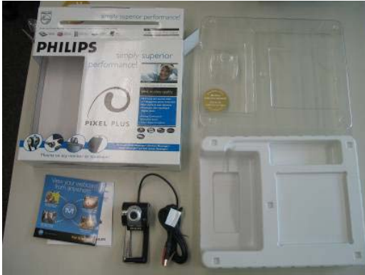
Figure 8.2: Unpacked web-cam. The contents (bottom right do not require this size of box. The size is purely a result of shelf performance considerations. (Pratama, 2006)
