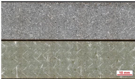
Fig. 10. Representative fracture surfaces from specimens tested at low temperature (crack growth direction to the right).
