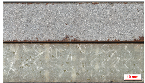
Fig. 15. Representative fracture surfaces from specimens tested after 222 days of aging (crack growth direction to the right).
