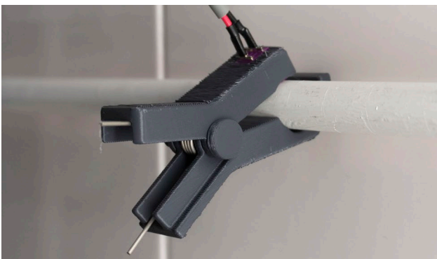
Figure 26. Clamp concept with stock part spring
