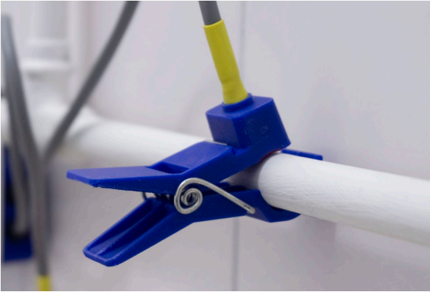
Figure 41. Use of a shrinking tube to finish the design
