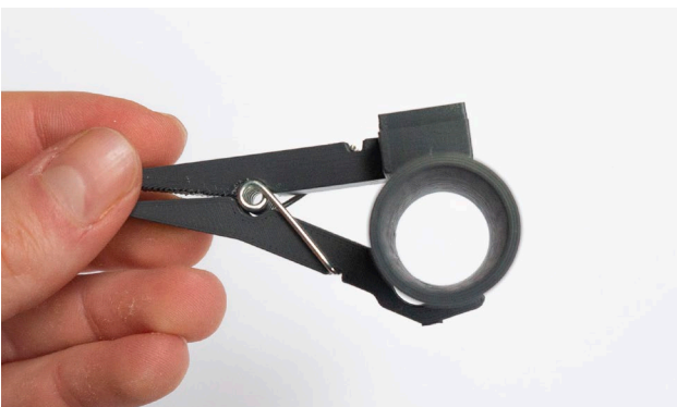
Figure 22. Clamp almost slipping off
