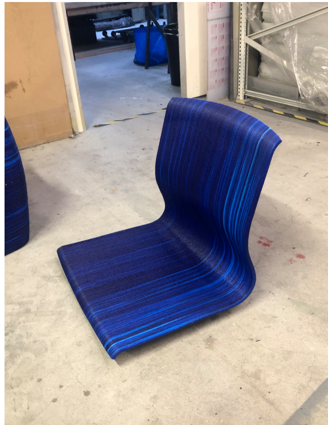
Figure 91: Finalized bucket chair shape after separating the print, refining and sanding the edges
