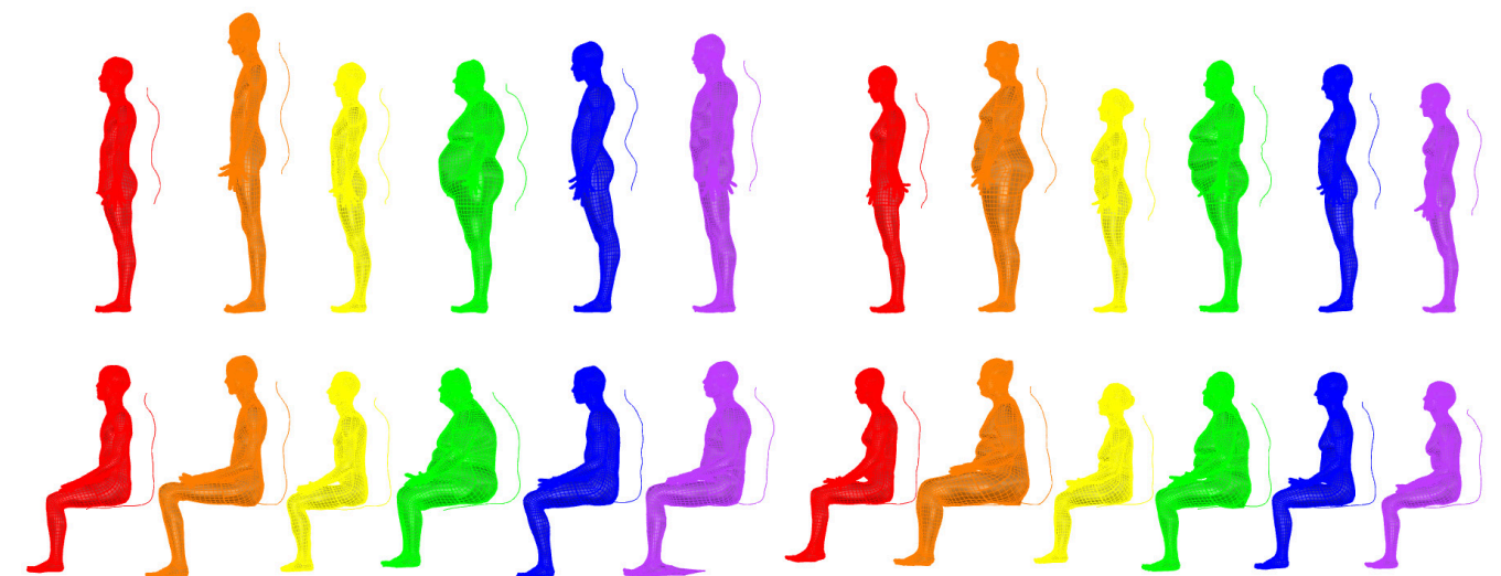
Figure 28: 12 different CAESAR models (left male, right female) with different body characteristics and their back curve measured
