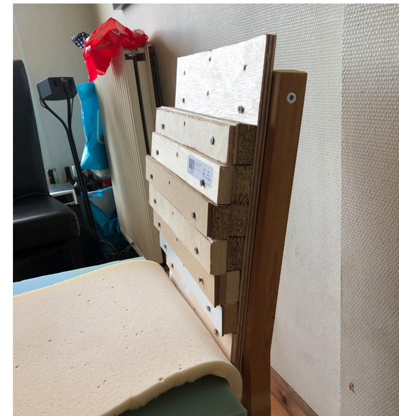
Figure 43: Prototype backrest with wooden slats of varying thicknesses
