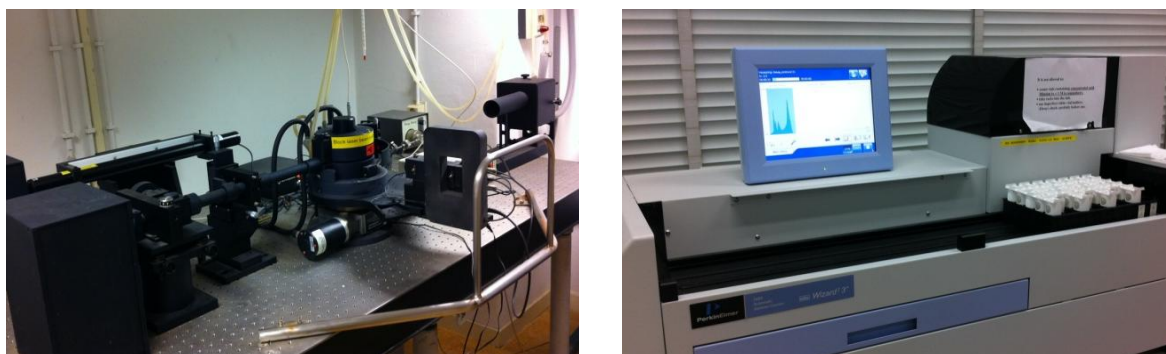
Figure 4.2 (Left) The dynamic light scattering apparatus with which size distributions and polydispersity of the polymersomes was assessed. (Right) A Wizard 2 Wallac 3'' 24800 Automatic Gamma Counter used for measuring activity in radionuclide containing samples. The energy spectrum of Indium-111 can be observed on the screen.
