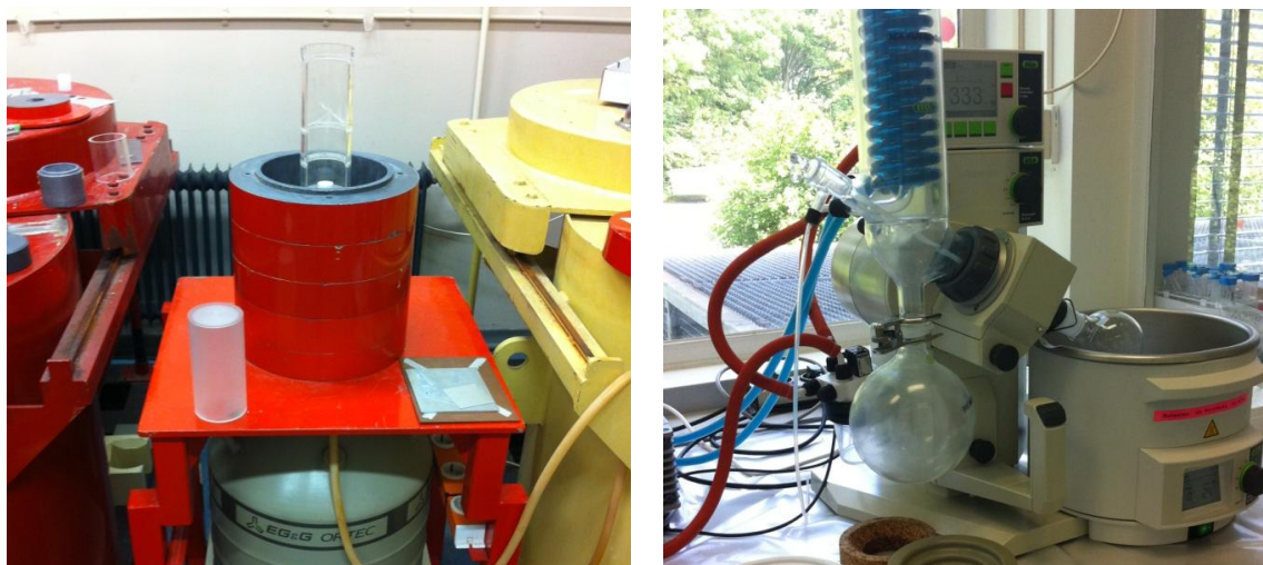
Figure 4.3 (Left) A LG22 High Purity Germanium (HPGe) detector from Gamma Tech used for measuring activity in radionuclide containing samples. (Right) A R-210 Rotavapor with a sample immersed in the corresponding B-491 heat bath.
