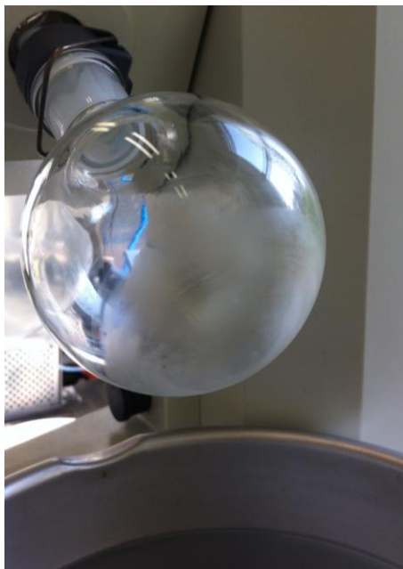
Figure 5.1 Preparation of a PCL130 sample by use of the BUCHI Rotavapor (M6). Upon evaporation of the organic solvent, a thin homogenous film can be seen to form on the flask.
