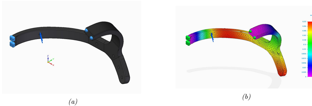
Figure 38: (a) Half of the halo is subjected for analysis and fixed on all 6 degrees of freedom on the plane of symmetry. The applied force is in longitudinal direction of the anterior pin. (b) Results of situation when 450 N is applied. The maximum displacement at this location is 0.16 mm
