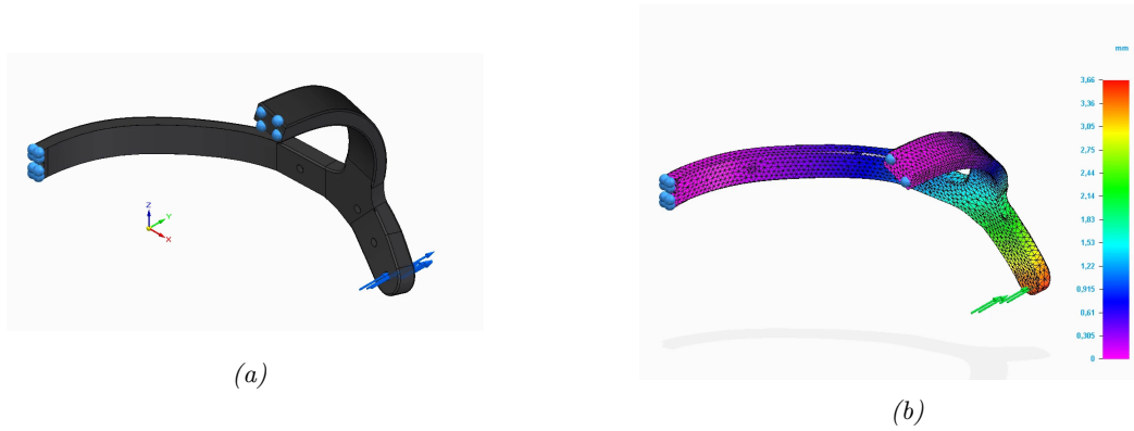
Figure 36: (a) Half of the halo was subjected to FEM analysis fixed on all 6 degrees of freedom in the plane of symmetry. The applied force was parallel to the 'y-axis' which was the same direction as the force applied in the experiments, as shown in Figure 33. (b) Displacements at a load of 450 N is applied. The maximum displacement was used in this analysis.
