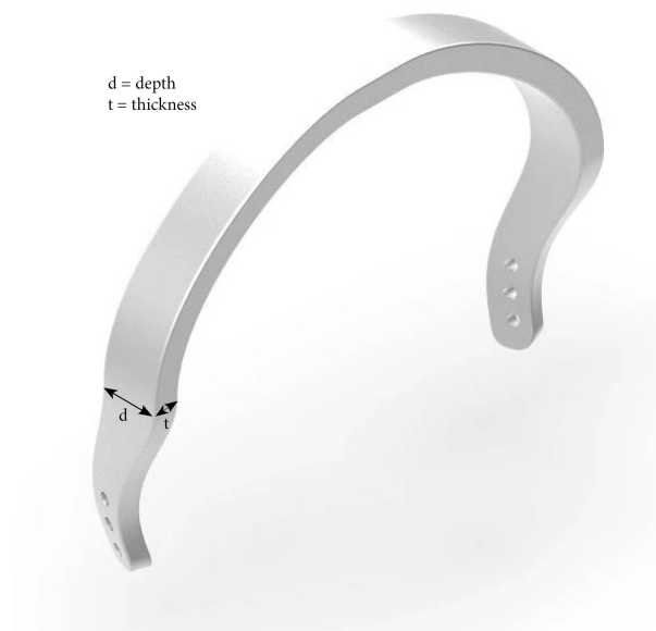
Figure 42: Thickness and depth of the posterior C-contour. The thickness and depth were not constant over the entire circumference of the C-contour. The variances between 't' and 'd' over the C-contour are partially determined by an optimization algorithm in Solid Edge ST10. The ratio between the variances were imposed by the designer. E.g. 't' inferiorly should always be smaller than 't' superiorly.
