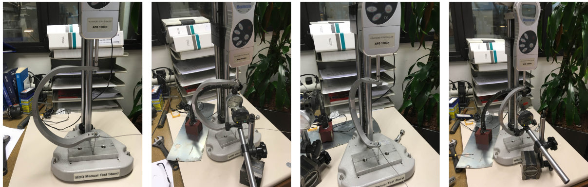
Figure 44: Overview of the test setup for measuring the stiffness at both the posterior and anterior pin sites.
