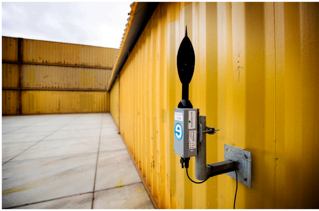
Fig. 3. Close-up of microphone 4 in front of a shipping container.
