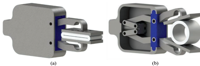
Figure 6-8: The 3D-model of the valve mechanism with the graft placed between the compressors. On the left it is shown without one of the side plates to expose the internal linkage, where the graft is in the fully open position with a relatively low transmission ratio in the linkage. On the right the side plate is shown, and the graft is fully closed. The design of the linkage creates a favorably high transmission ratio in this position to fully close the graft. Models were made in SolidWorks (Dassault Systèmes, Paris, France).
