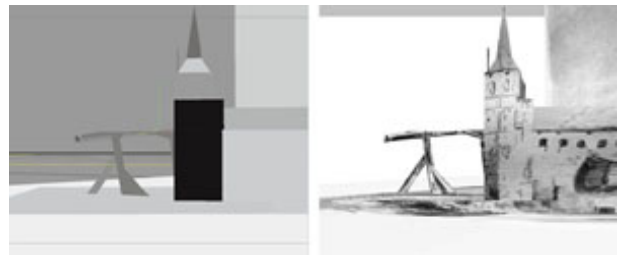
Wireframe of a newly created perspective (on the left): a side view of the Rotterdam Gate. In the image on the right, the corresponding textures have been applied.
