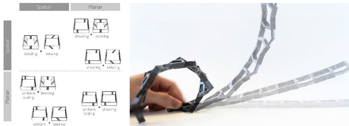
Figure 9: Spatial transformation includes bending and twisting. Combining these can achieve desired transformation (Ou et al., 2018)
