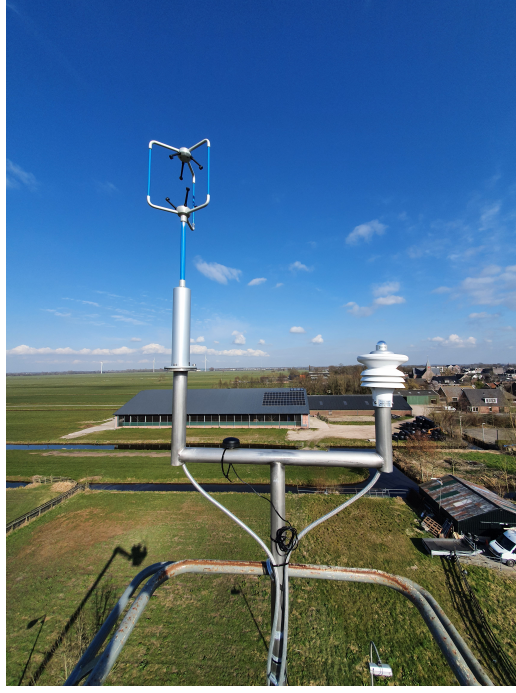
Fig. 7: Turbulence monitor placed on top of crane with sonic anemometer on the left side of the T-post.
