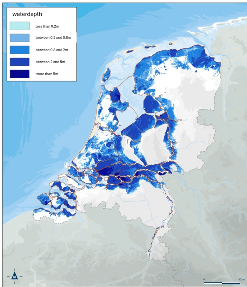
Figure 1.5.: Overview of the flood prone are in the Netherlands, based on the flood simulations in the National database flood simulations [54, 55].
