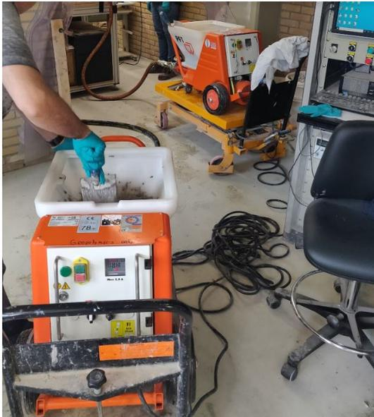
Figure 5.5: Two material conveying pumps with separate pumping hoses
