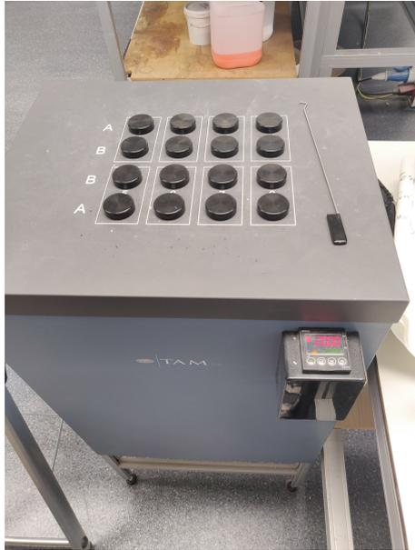
Figure 5.4: TAM Air calorimeter with eight channels
