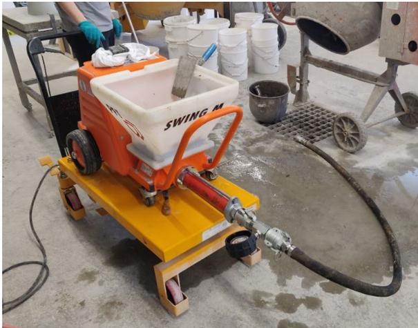
Figure 5.1: Test set-up of the material conveying pump
