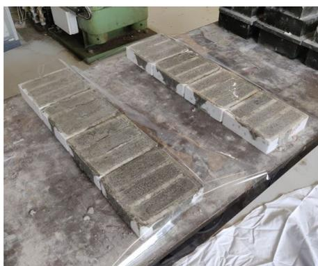
(a) Plastic film for curing of the mortar
