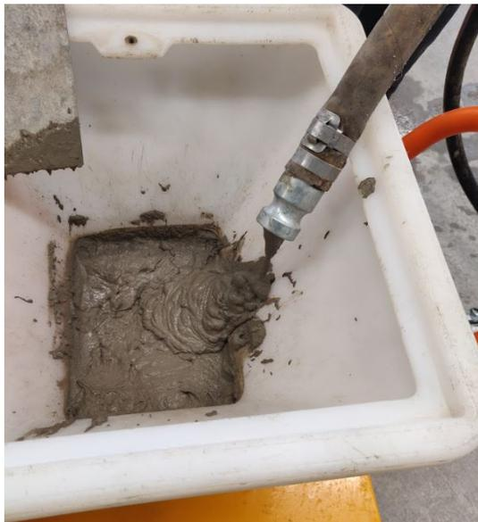
Figure 5.3: Pumpability test material pumping
