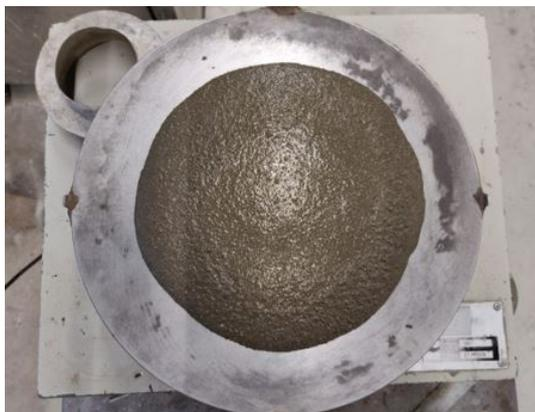
Figure 3.18: Slump flow test after 25 drops of the compaction table
