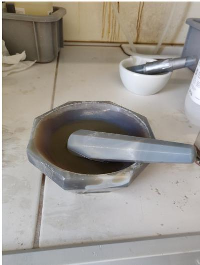
Figure 4.1: Grinding the paste to a powder in isopropanol
