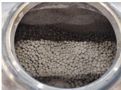
Figure 3.9: Fine glass dust with milling balls
