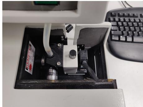
(b) Lens and laser for PSD
