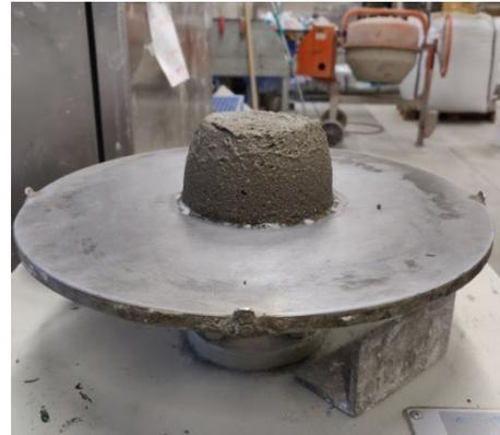
(b) Slump test after removing the mould
