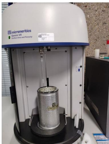
Figure 3.11: Micromeritics Gemini VII for BET analysis
