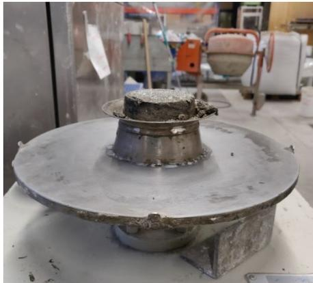
(a) Filled mould for the slump test
