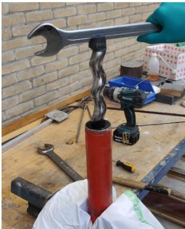
(a) Rotor-stator system
