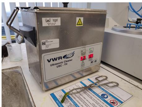
Figure 3.2: Ultrasonic cleaner for preparation of PSD samples
