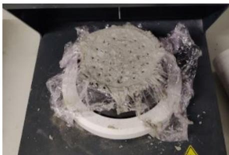
Figure 3.21: Finished Vicat test
