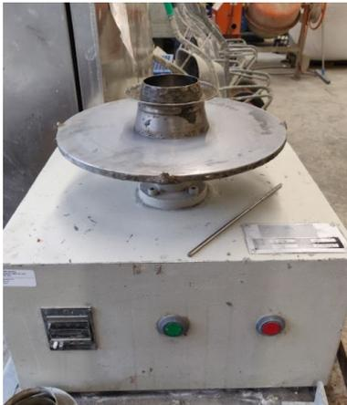
Figure 3.16: Set-up on compaction table for mini slump test
