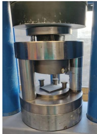
(b) Loading jig for compressive strength test
