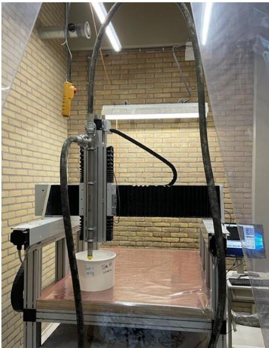
Figure 5.6: Helical static mixer set-up with printing nozzle (Yu Chen)
