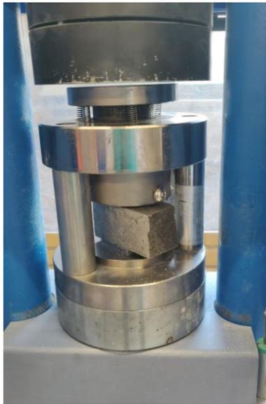
Figure 3.24: Loading jig with sample for compression test
