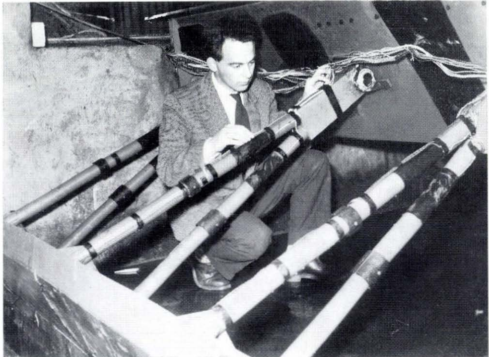
A model being used for research into wave impact on segmental gates
