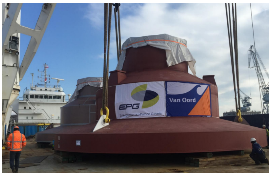
Figure 1.3: Spudcan design of the Aeolus [21].
