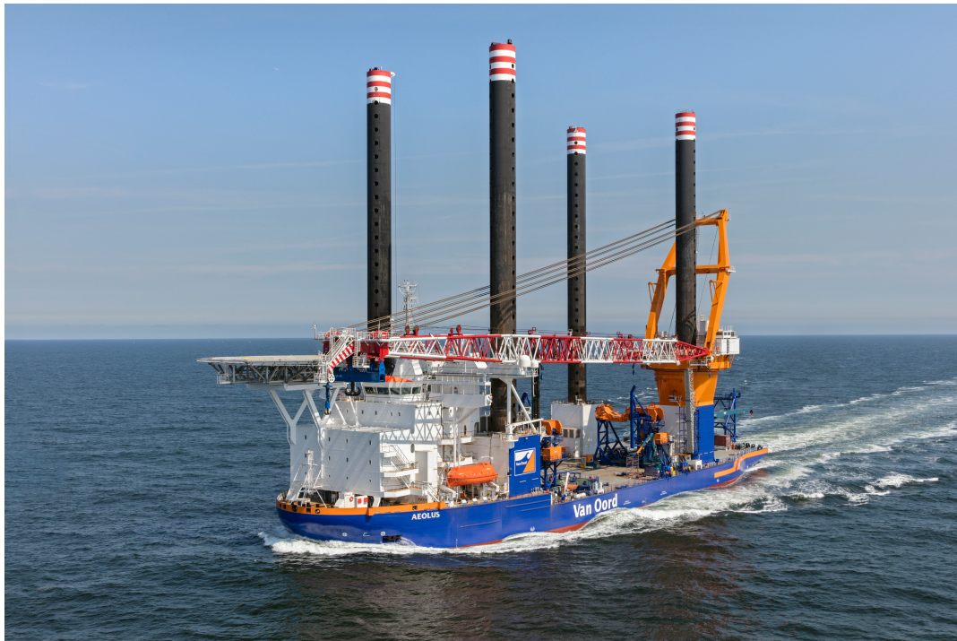
Figure 1.2: The offshore jack-up installation vessel Aeolus with the old crane boom [8].
