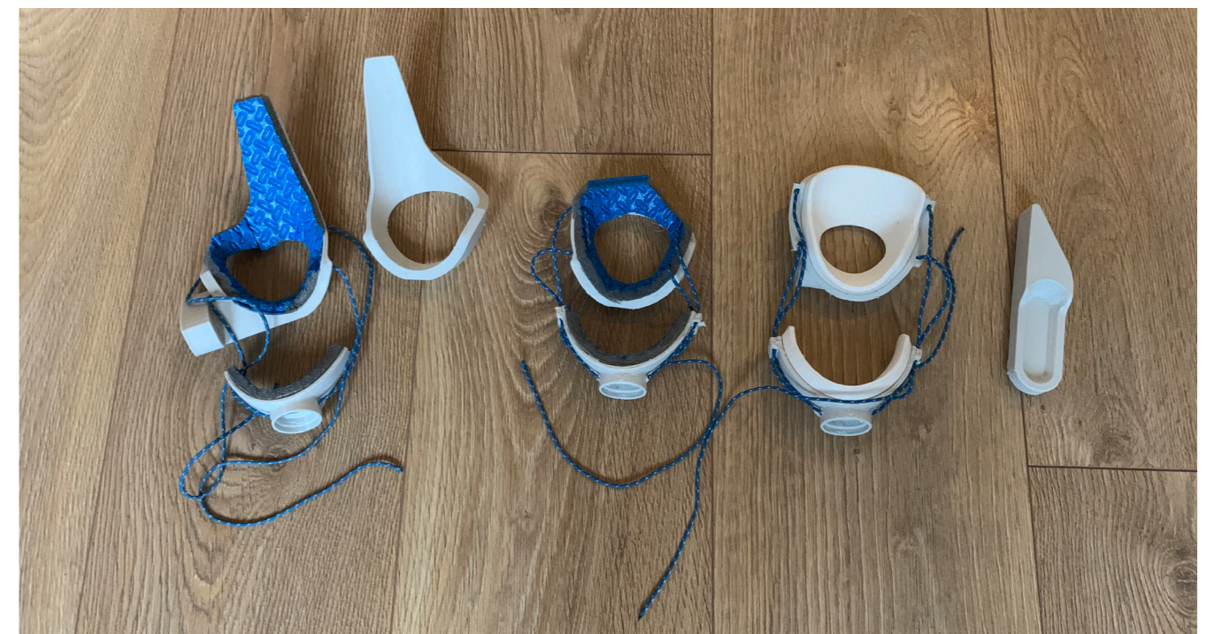
Fig. 70 - 3D printed heel cup and cable system iterations
