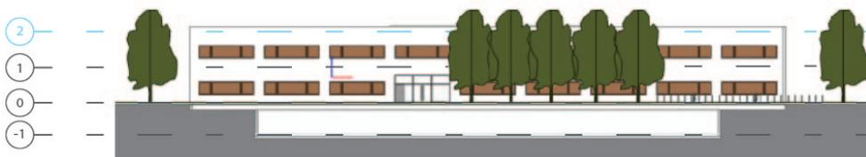
Figure 5.2.: Example of the roof storey that is added by the tool. The gray storey elevations were already present in the original IFC file of the DigitalHub model. It can be seen that the roofing structure of the model has no dedicated storey elevation. This elevation, highlighted in blue, is added by the tool.
