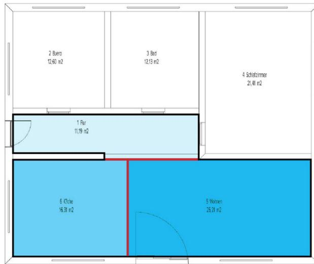
Figure 5.27.: Floorplan of the ground floor of the FZK-Haus model with the three *IfcSpace* shapes, occupying the largest space, highlighted. The faces of each *IfcSpace* shapes that rests against another is highlighted. These connections can not be detected by the tool.
