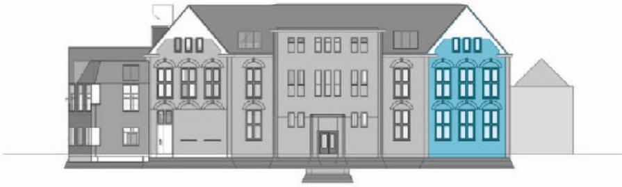
Figure 5.12.: The *Witte\_de\_Withstraat* model with a wall highlighted that is labelled to be on the first floor instead of the ground floor. This is caused by picking the basepoint for the elevation of a wall at a third of its height. This is very high for walls spanning multiple floors.
