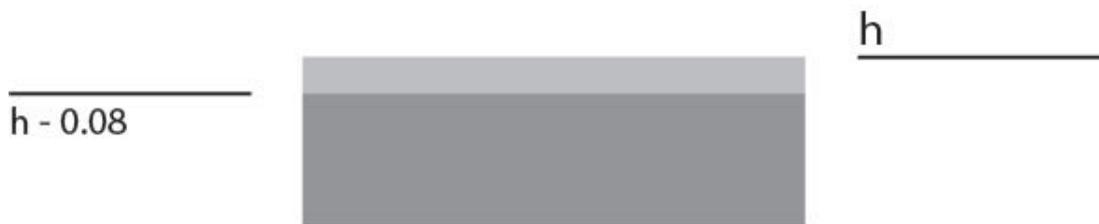
Figure 5.6.: The situation in the *Boompjes* model that creates an undesired z-value extraction. The flooring is constructed out of a structural floor (dark gray) and a screed floor (light gray). Even when both are evaluated by the tool, the tool will merge the z-values found in these floors to the lowest of the tool, resulting in the z-value still being 8 cm lower than expected.
