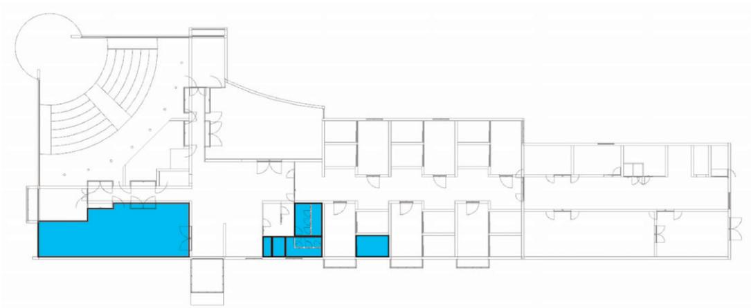
Figure 5.28.: The room clusters incorrectly considered by the tool to be connected to the outside
