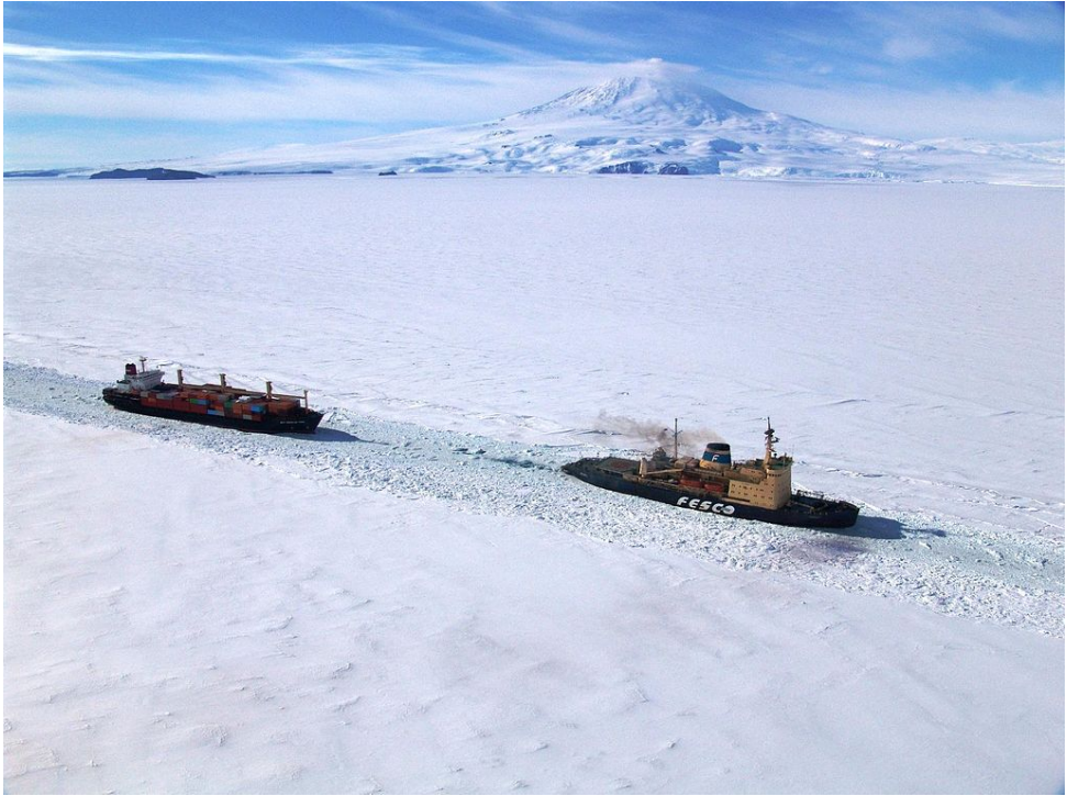
Figure 1.3: Russian icebreaker Krasin leading an American supply ship through level ice during Operation Deepfreeze in 2006. Image courtesy: NSF.
