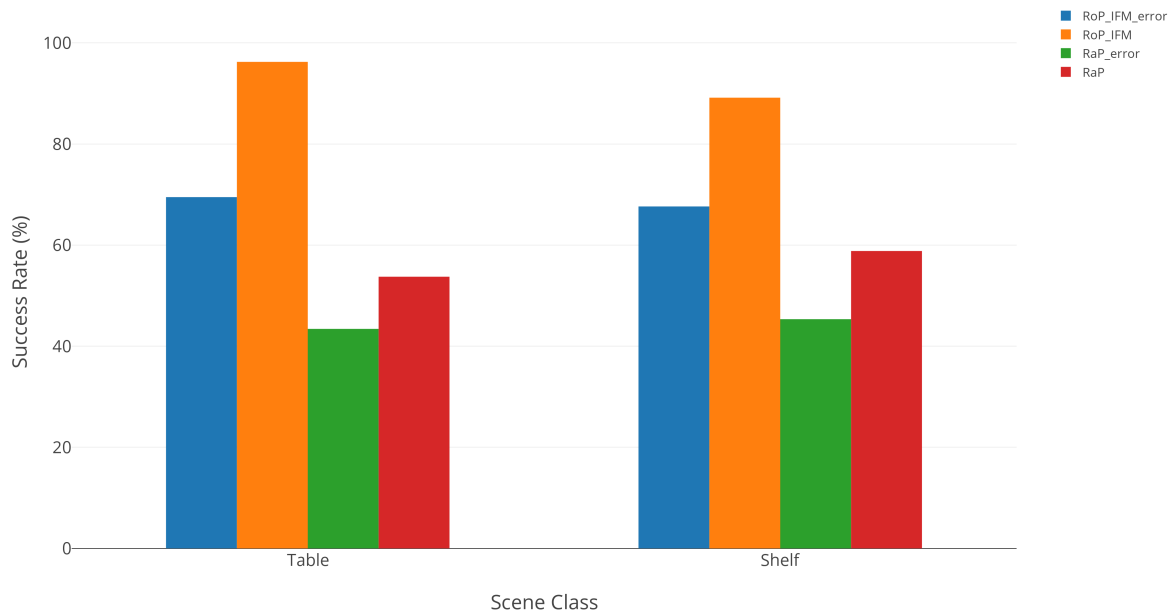
Figure 5-11: Average success rate in planning to targets on Table and Shelf in presence of actuation uncertainty. Introduction of actuation error reduces the success rate, yet performance remains better than random placement
