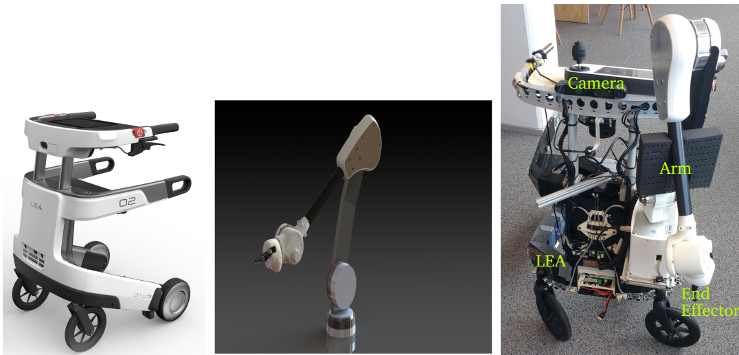
Figure 1-2: Model of LEA mobile base (left), and 6 d.o.f. arm (center), LEA with arm prototype.
