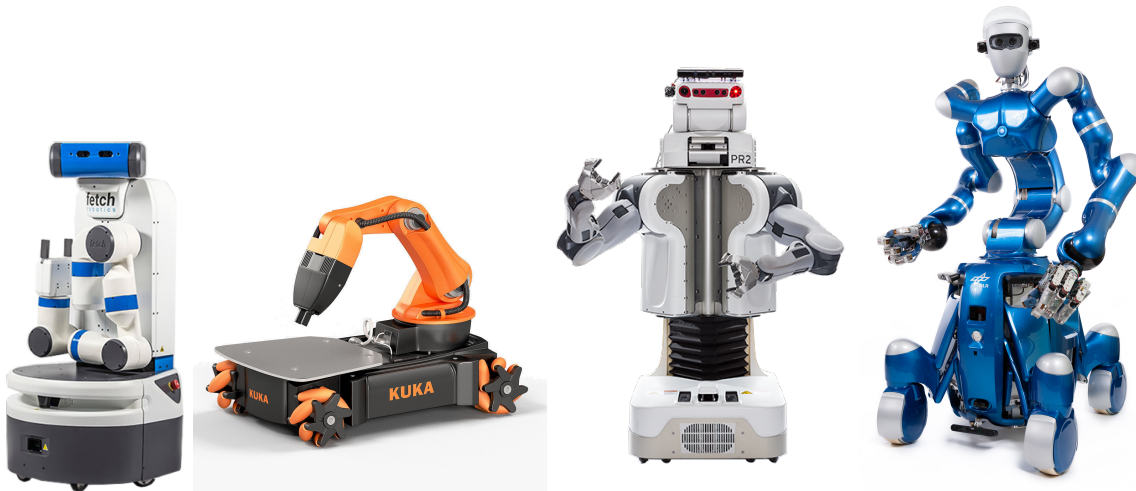
Figure 1-1: State-of-Art Mobile Manipulators(from left to right): FETCH [13], KUKA Youbot [14] , PR2 [15], Rollin' Justin [16]
