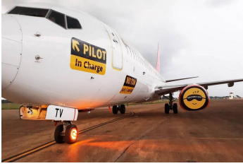
(a) The WheelTug, an example of an internal towing system [53]. (b) The TaxiBot, an example of an external towing system (an ETV)[54].
