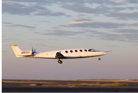
Figure 1.4.: The Eviation Alice, the first 10 passenger pure-electric aircraft (image: Eviation).
