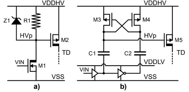
Fig. 3. Level shifter architectures based on a) HV transistors and b) capacitors.
