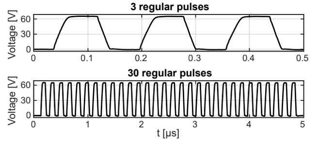
Fig. 6. Electrical measurement of 3 and 30 pulses from the proposed pulser.
