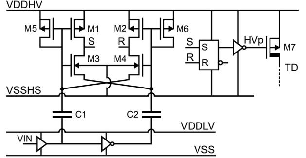
Fig. 4. Proposed supply transient insensitive, capacitor-based HV level shifter.
