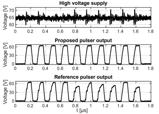
Fig. 7. Comparison of pulsing with the proposed and reference HV level shifter in the presence of supply ripple with 27 nH added supply inductance.
