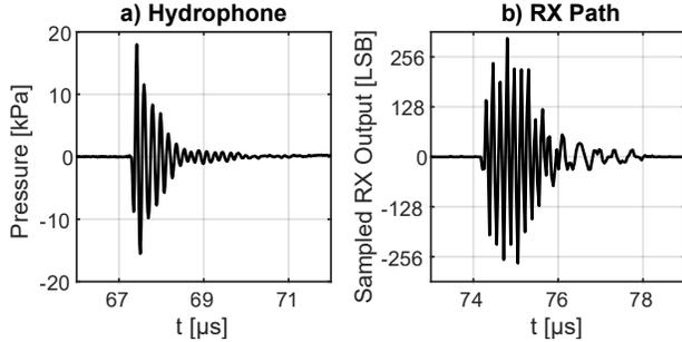
Fig. 9. One transmitted pulse measured by a hydrophone at about 10 cm distance in a) and reflected at about 5.5 cm from plate-reflector, received by the on-chip analog frontend and sampled at 24 MHz in b).
