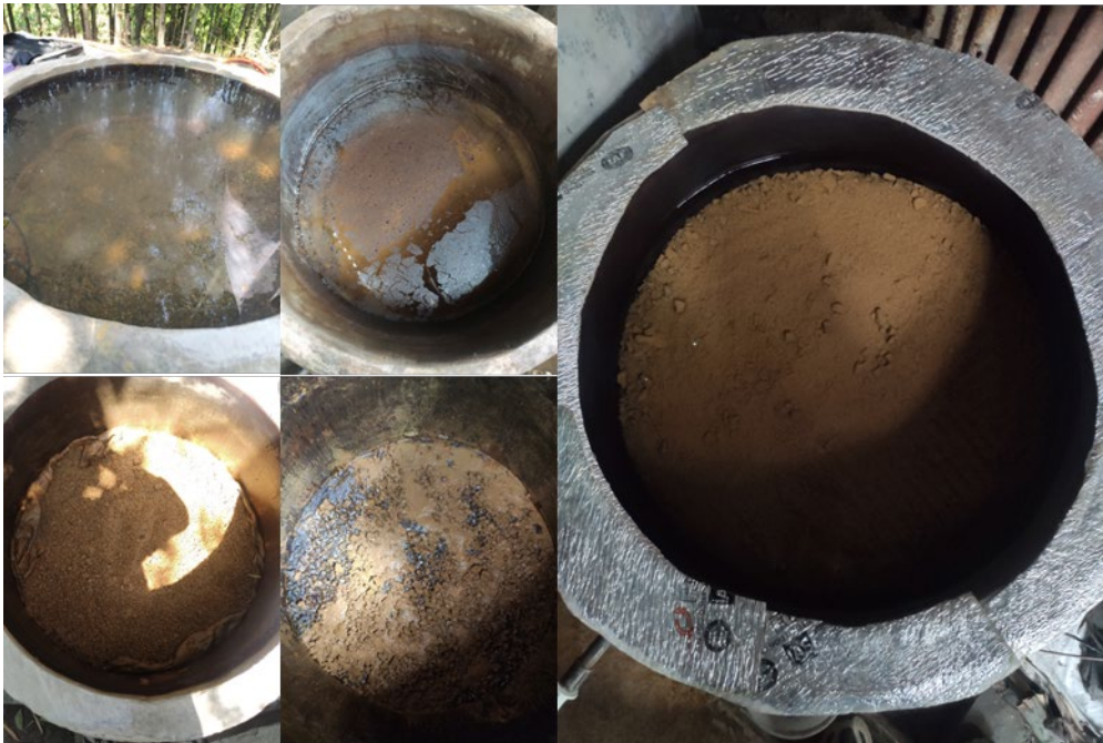
Figure S4: Pictures of Fe flocs present in the effluent of the tank at H1 (left two) H2 (middle two) and H3 (right). Both flocs floating in the water (top pictures), as flocs precipitated on the top of the filter bed (bottom and right pictures) are visible. Note: the filter is upflow, so the supernatant water is the treated effluent.
