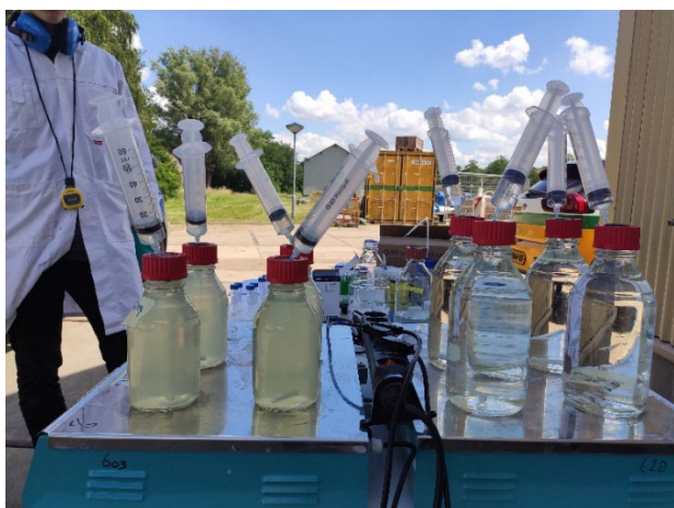
Figure 1: Picture of batch experiments using anaerobic concentrate (4 bottles left) and anaerobic groundwater (four bottles right) as performed on site TP1 & TP2.
