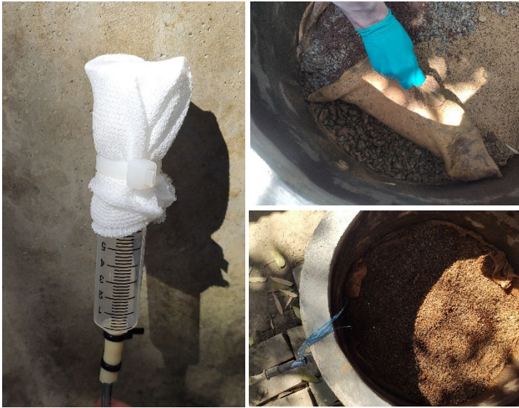
Figure S3: Pictures of the sampling setup of taking the vertical removal profile at household-scale treatment plants H1-H3. Left: the syringe and filter sock which was placed in each different filter layer (right top). Right bottom shows how the three tubes coming out of the bed after placing back the layers.
