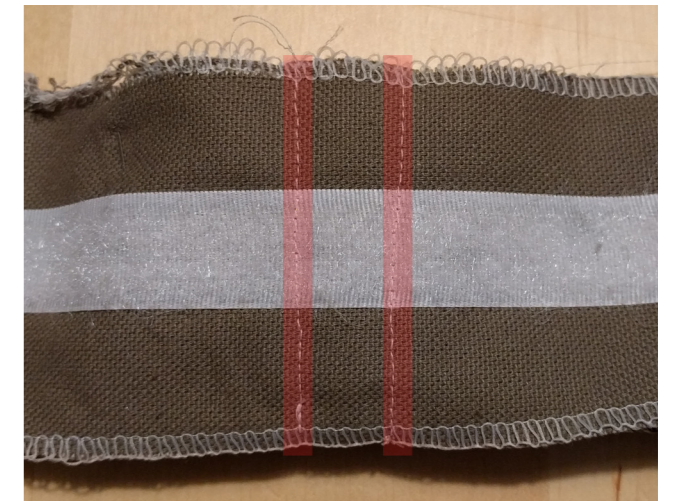
Figure 45. Every 50 cm has closed stitch so the user can cut if they need to
