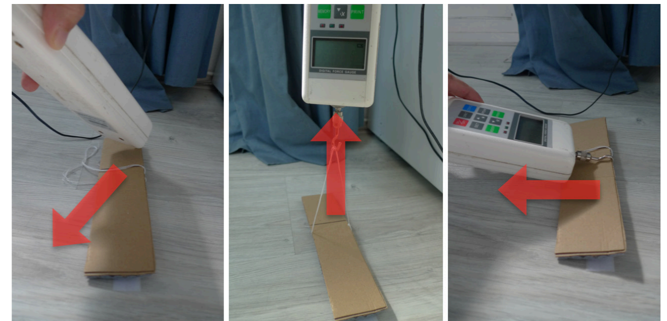
Figure 43. Solidity test (from left: Diagonal, up, and side direction)
