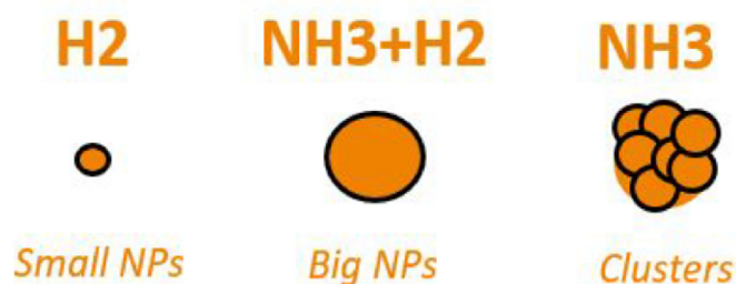
Fig. 4. The catalyst NP determined by the three annealing gases (H 2 , H 2 + NH 3 , NH 3 ). (A colour version of this figure can be viewed online.)
