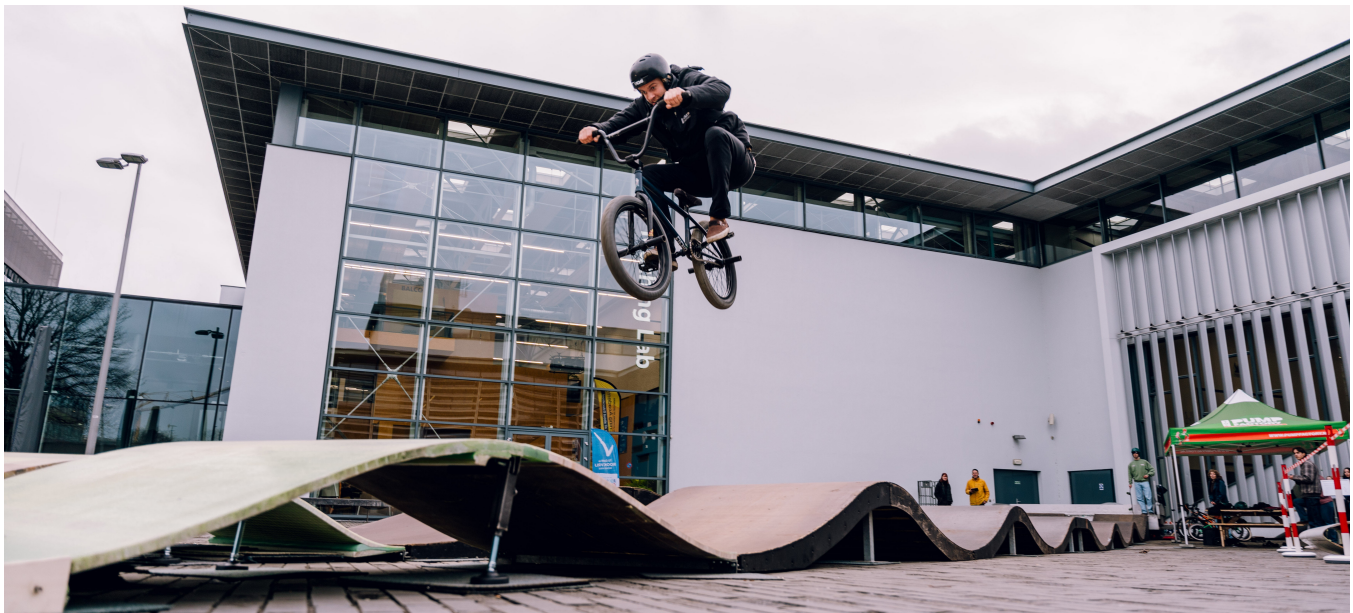
Figure 1: Our prototype pumptrack module (seen on the left hand-side of the picture) being tested by a BMX rider. Our module is made of two panels extracted from a decommissioned wind turbine blade, and matches the curvature of standard modules (seen on the right hand-side). Picture by ©Patrick Wetzels, TU Delft.
