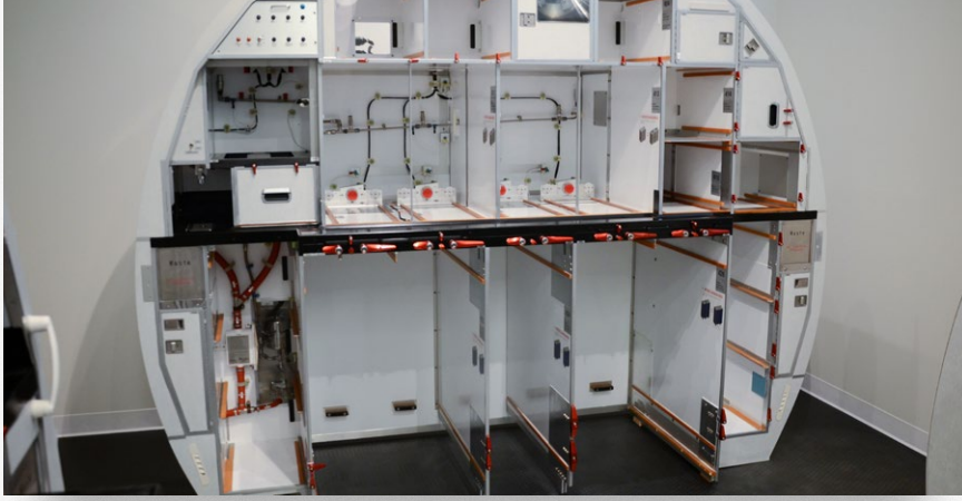
Fig.100 An empty Boeing 737 galley storage area from Jamco (Ostrower, 2014)
