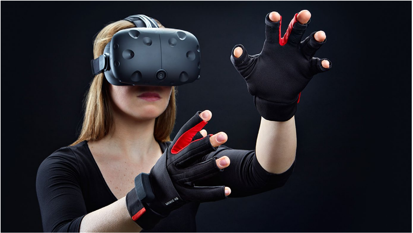
Fig.43 Manus VR does hand tracking with integrated sensors (Manus VR, 2015)
