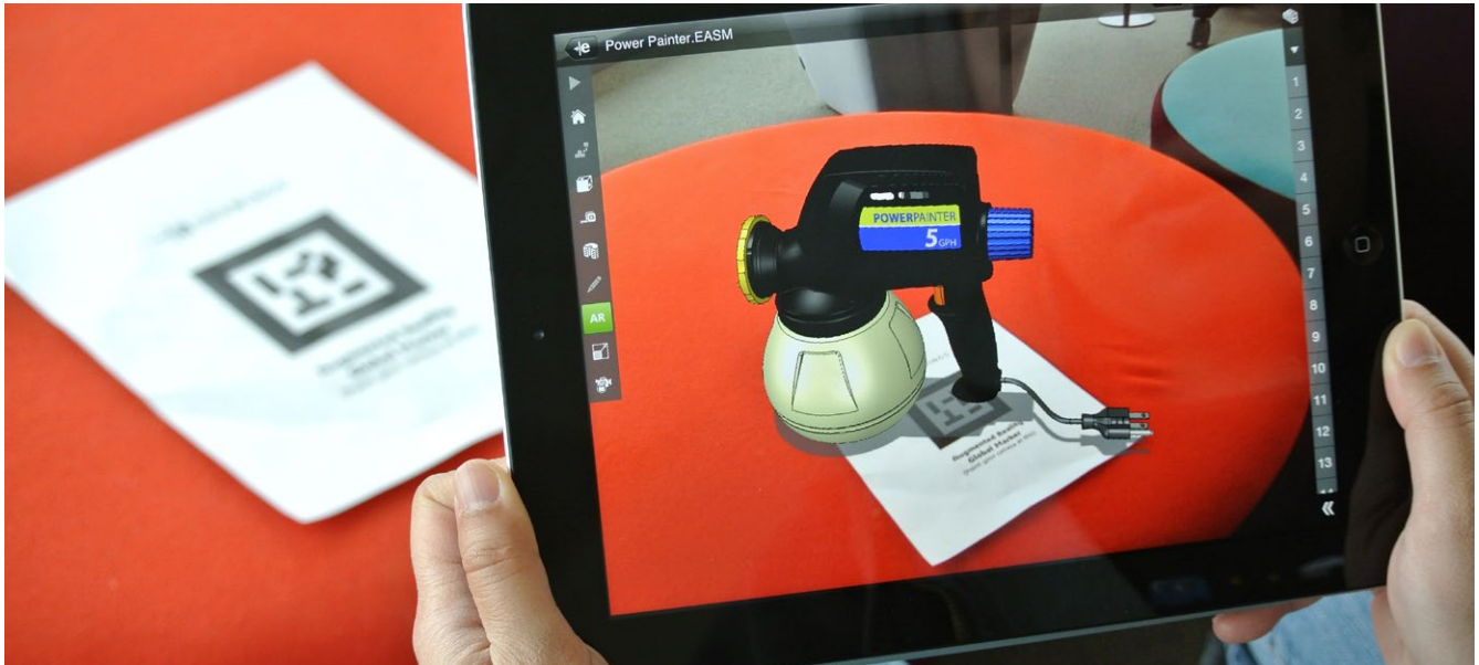
Fig.38 Handheld AR using camera overlay and tracking marker (Chin, 2013)
