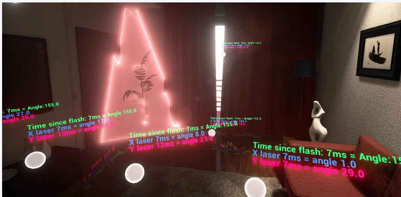
Fig.42 HTC Vive Lighthouse system working principle (van der Meer, 2015)
