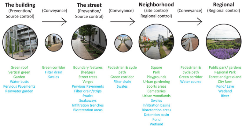
Figure 23: Green Infrastructure and SUDS through the scales (Scottish government, 2011)(Woods-Ballard et al., 2007).
