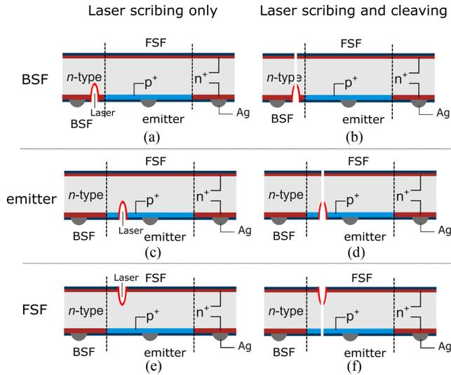
Fig. 1. Schematic structure (not to scale) of cells with different cutting scenarios. (a) and (b) BSF group: Cuts on BSF and cleaved through the BSF region. (c) and (d) Emitter Group: Cuts on emitter and cleaved through the emitter region. (e) and (f) FSF Group: Cuts on FSF and cleaved through the emitter region.
