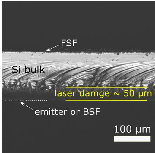
Fig. 5. Cross-section of the laser cutting area.
