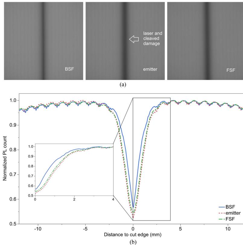
Fig. 7. (a) PL images of the laser cut regions after laser cut and cleaving, with the same scaling. From left to right-hand side: BSF, emitter, and FSF. (b) Cross-section of PL profiles from the cell edge.
