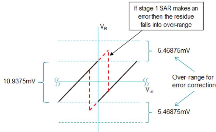
FIGURE 2.4: Over-range to correct the error from first stage of the pipelined SAR-ADC
