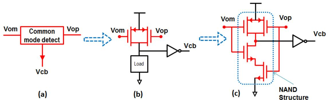
FIGURE 4.10: The concept for common-mode detect circuit
