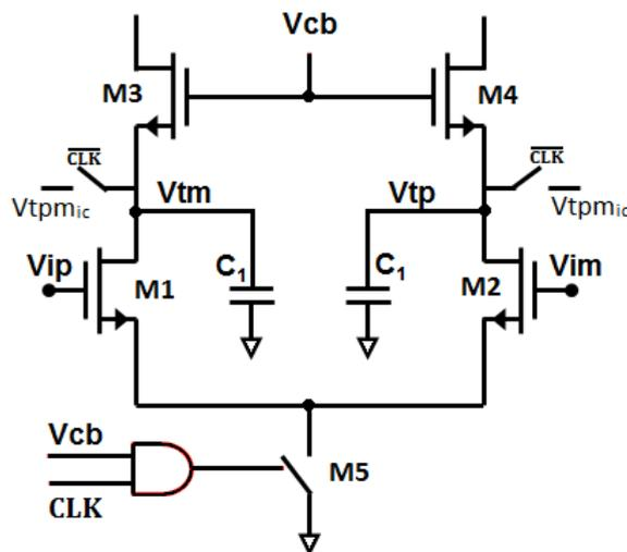
FIGURE 6.1: Input pair and cascode pair of CIDRA
