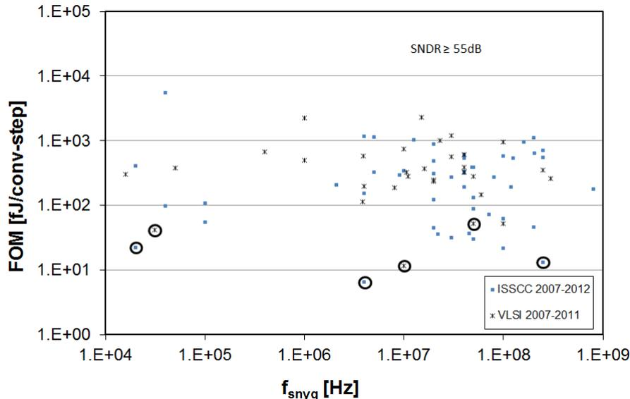
FIGURE 1.1: Figure of merit (FoM) versus Nyquist frequency ( $f_{\text{snyq}}$ ) of recently published ADCs with  $\text{SNDR} \geq 55$  [2]
