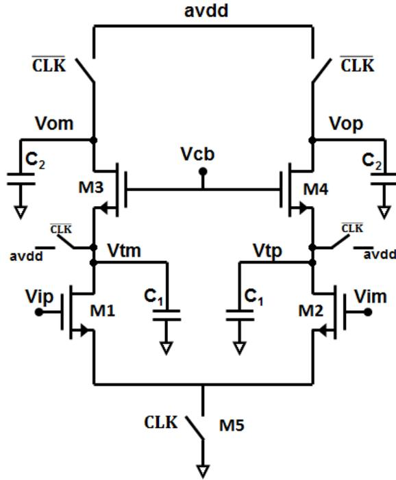
FIGURE 4.3: Cascoded integrator
