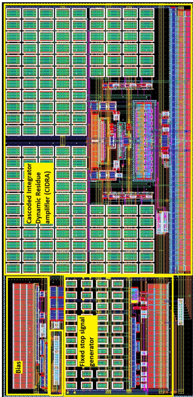
FIGURE B.1: CIDRA : Layout, and the size (width,height) of this module is  $(85\mu\text{m}, 41\mu\text{m})$
