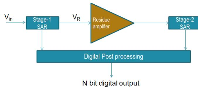
FIGURE 1.2: Block diagram of pipelined SAR-ADC
