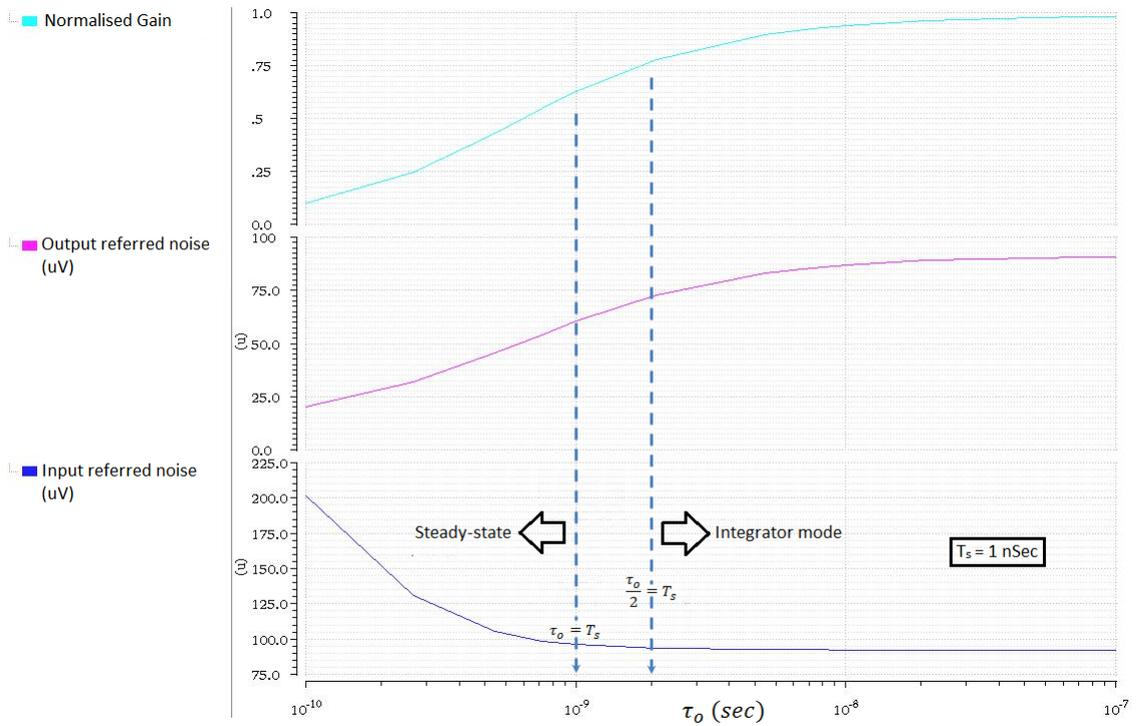
FIGURE 3.5: Gain, output referred noise and input referred noise versus  $\tau_o$
