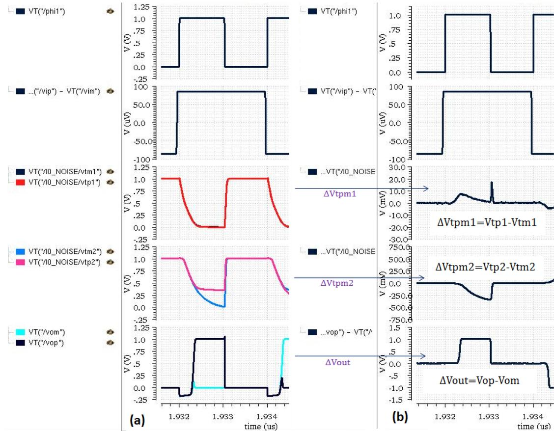
FIGURE 5.4: A transient decision cycle of the PLPDC of Figure 5.3 (a) individual node voltages (b) differential voltages
