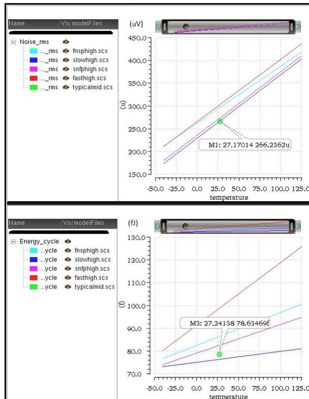
FIGURE A.8: Comparator-2 : Temperature and Corner simulations results of Noise(input referred) and Energy/cycle
