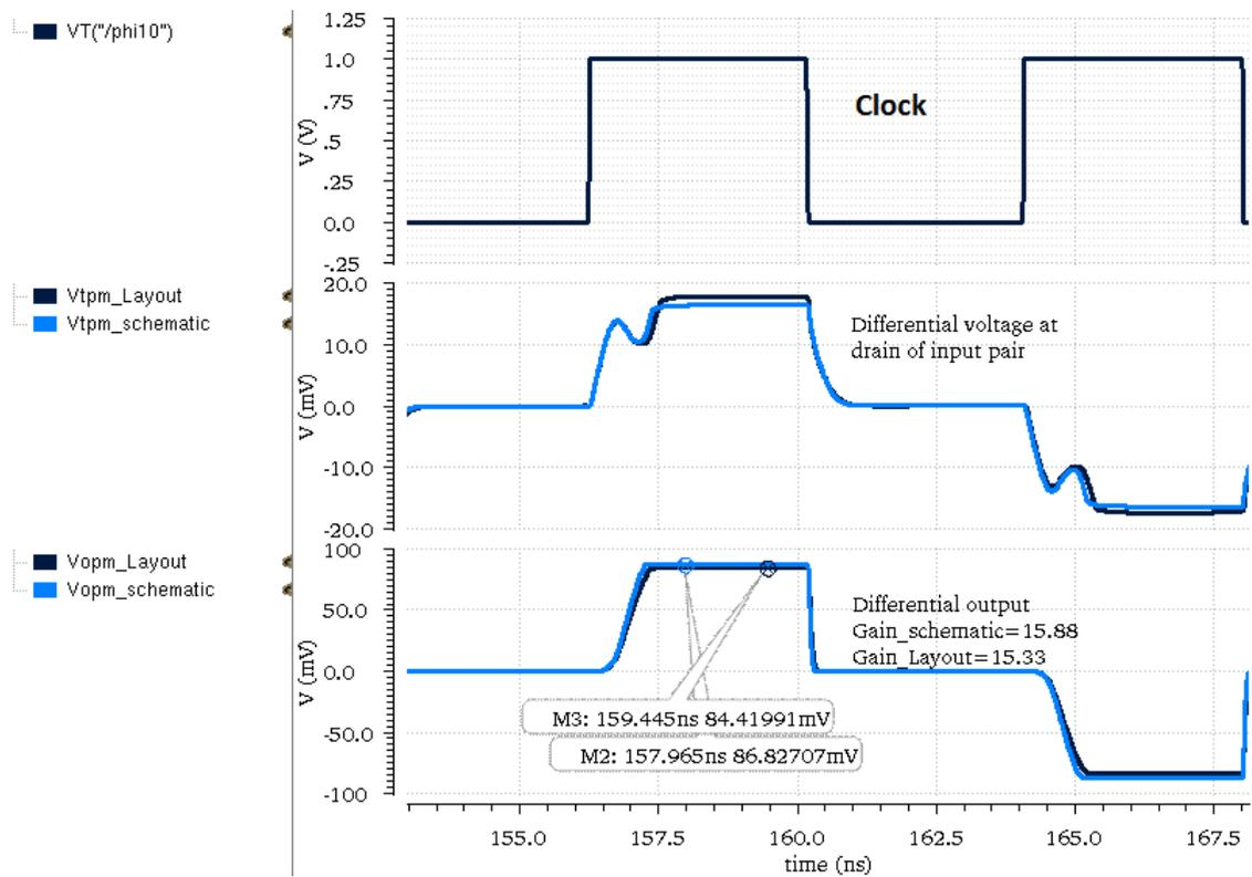
FIGURE B.4: CIDRA : Differential voltage at drain of input pair and differential output of schematic and post layout simulations
