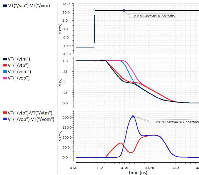
FIGURE 4.9: Simulation of the cascoded integrator of Figure 4.3 (see Table 4.1 for parameters)
