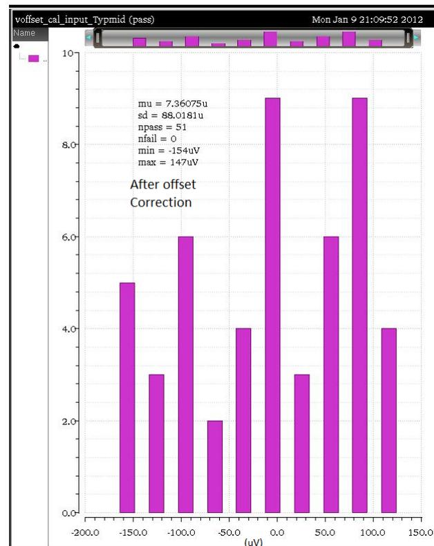
FIGURE A.5: CIDRA : Input referred offset after correction
