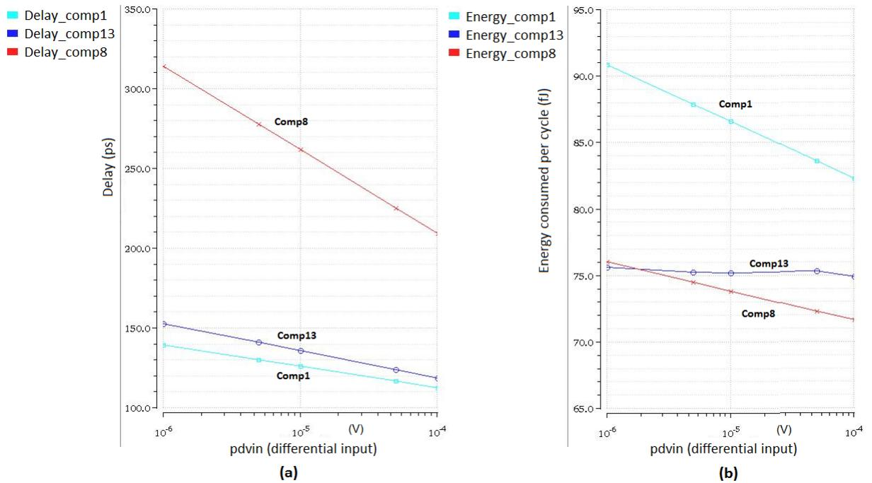
FIGURE 5.6: All the three comparators designed with similar transistor sizes (comp1=Sense amplifier; comp8=Double-tail comparator; comp13=PLPDC) (a) Delay vs differential input voltage (pdvin) (b) Energy consumed vs differential input voltage (pdvin)
