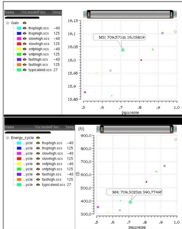
FIGURE A.1: CIDRA : Temperature and Corner simulations results of Gain and Energy/cycle
