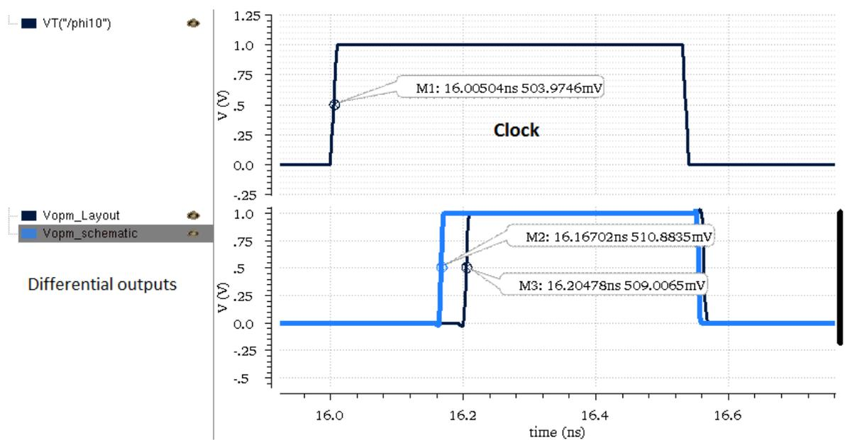
FIGURE B.5: PLPDC-1 : Differential output voltage of schematic and post layout simulations
