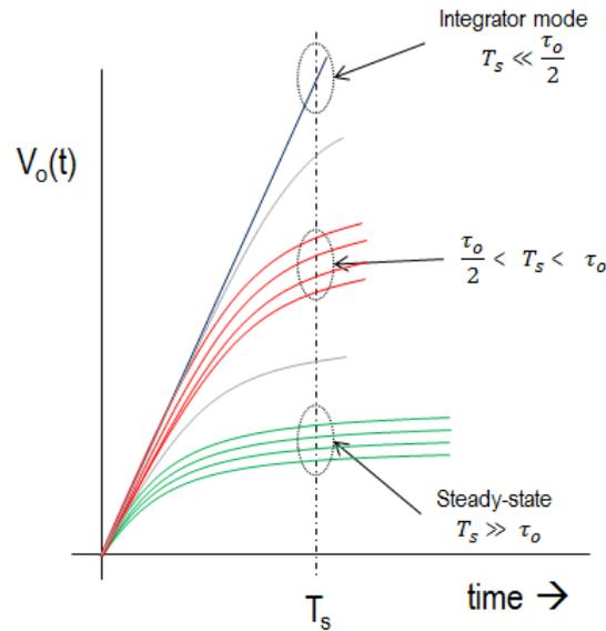
FIGURE 3.3: Step response of transconductance amplifier versus time for different time constant  $R_o$  values ( $\tau_o = R_o C$ )
