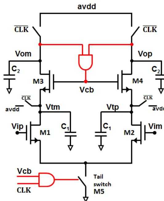
FIGURE 4.11: Cascoded integrator dynamic residue amplifier (CIDRA)
