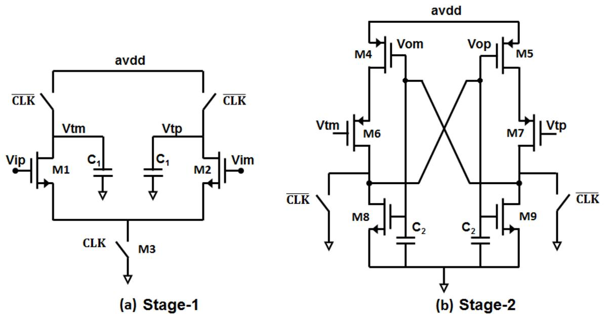
FIGURE 5.2: Double-tail comparator (a) Stage-1 (b) Stage-2
