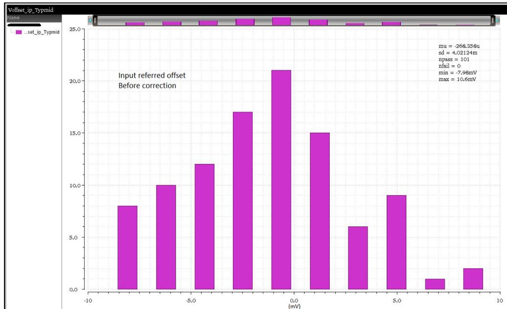
FIGURE A.10: Comparator-1 : Input referred offset before correction
