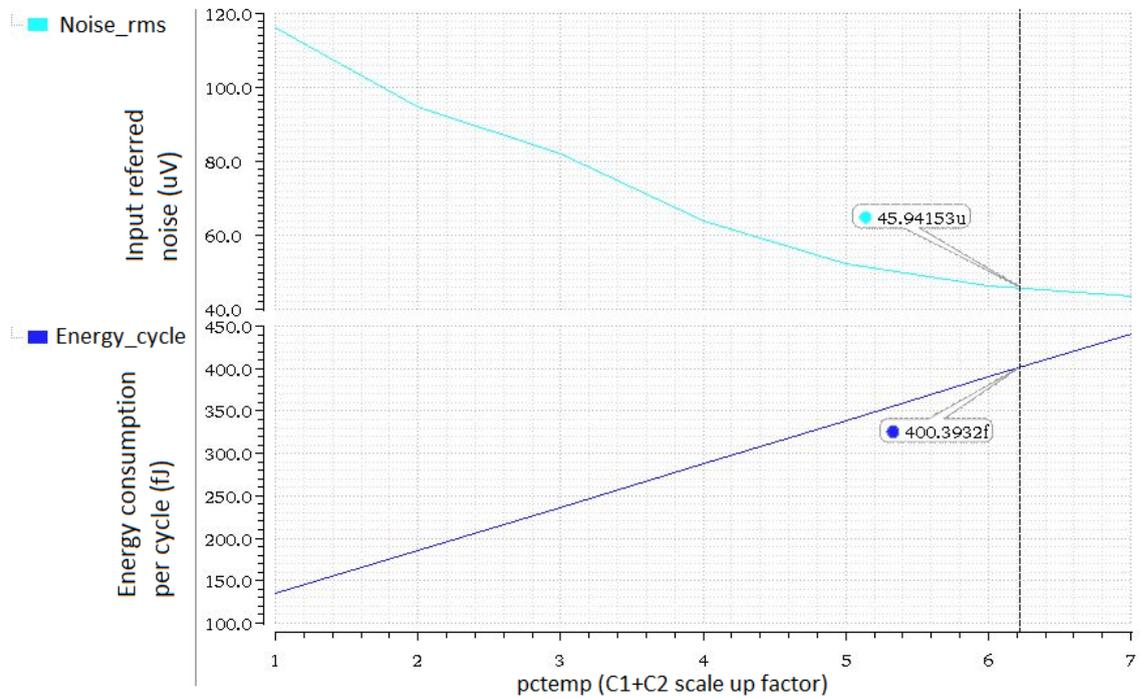
FIGURE C.1: The input referred noise and the energy consumption of a sense amplifier based comparator
