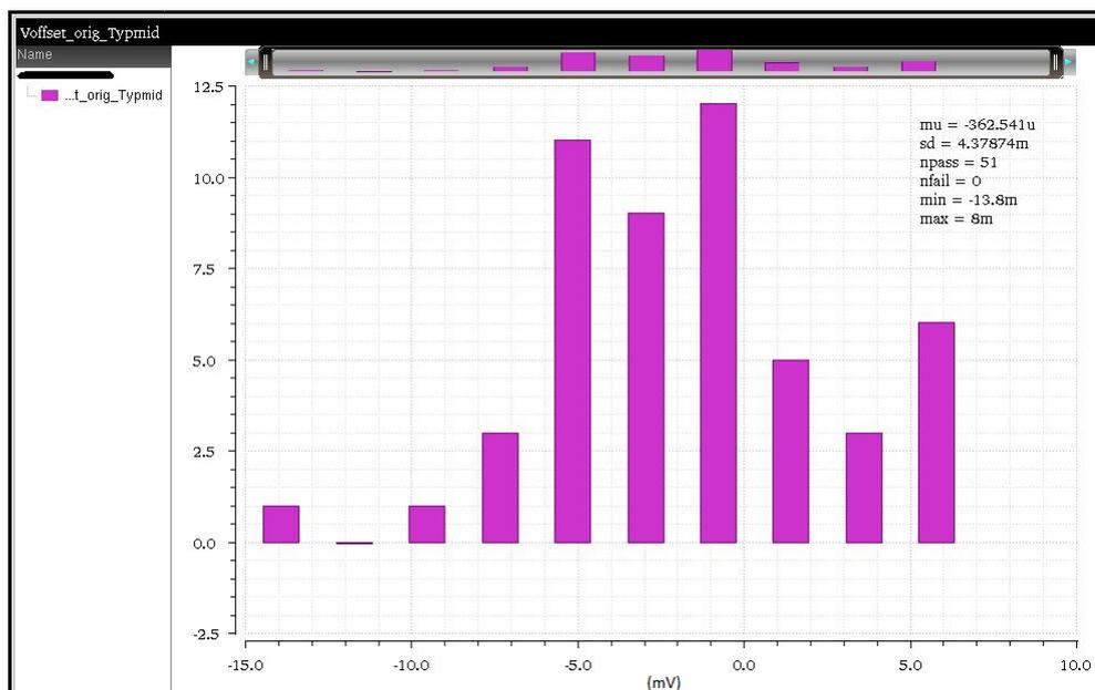
FIGURE A.13: Comparator-2 : Input referred offset before correction
