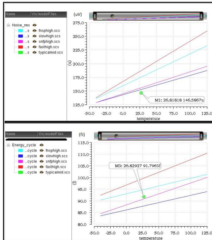
FIGURE A.6: Comparator-1 : Temperature and Corner simulations results of Noise(input referred) and Energy/cycle
