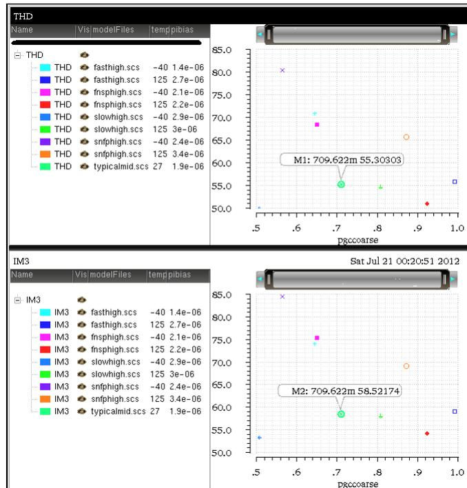
FIGURE A.3: CIDRA : Temperature and Corner (two tone) simulation results of THD and IM3
