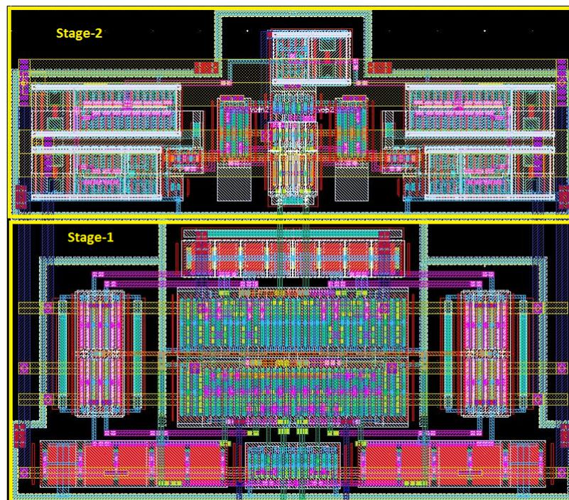
FIGURE B.2: PLPDC-1: Layout, and the size (width,height) of this module is  $(12\mu\text{m},11\mu\text{m})$
