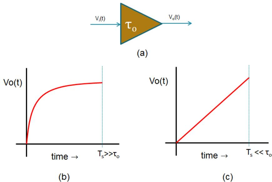
FIGURE 3.1: Step response of transconductance amplifier (a) Transconductance amplifier with time constant  $\tau_o$ (b)steady-state mode response (c) integrator mode response
