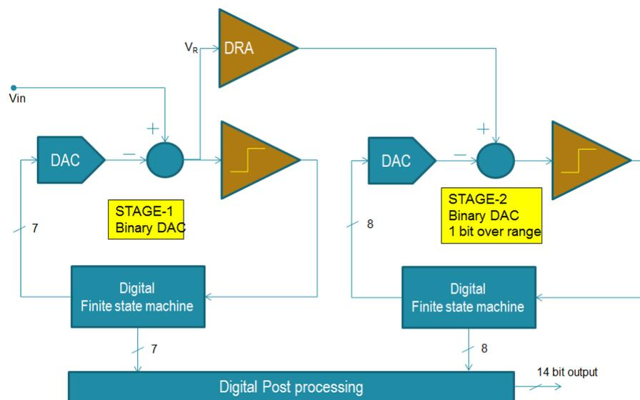
FIGURE 2.2: 14-bit pipelined SAR architecture
