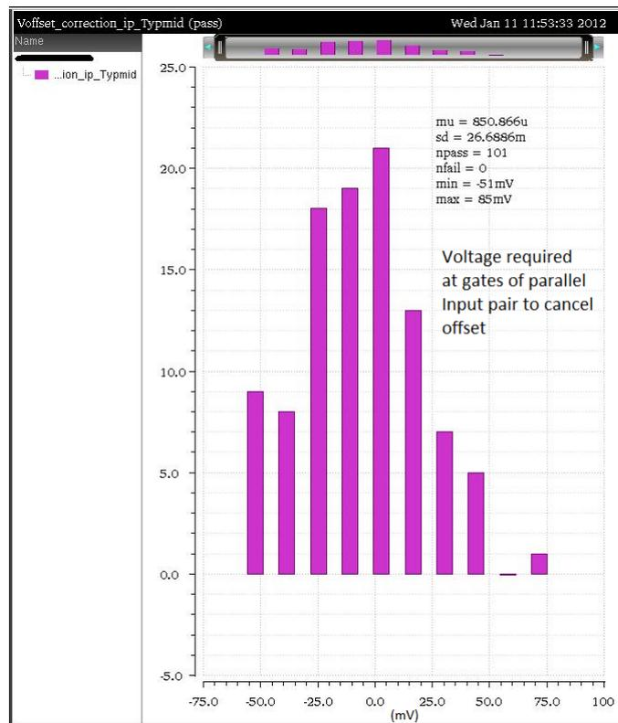
FIGURE A.12: Comparator-1 : voltage at gate of parallel input pair to cancel offset
