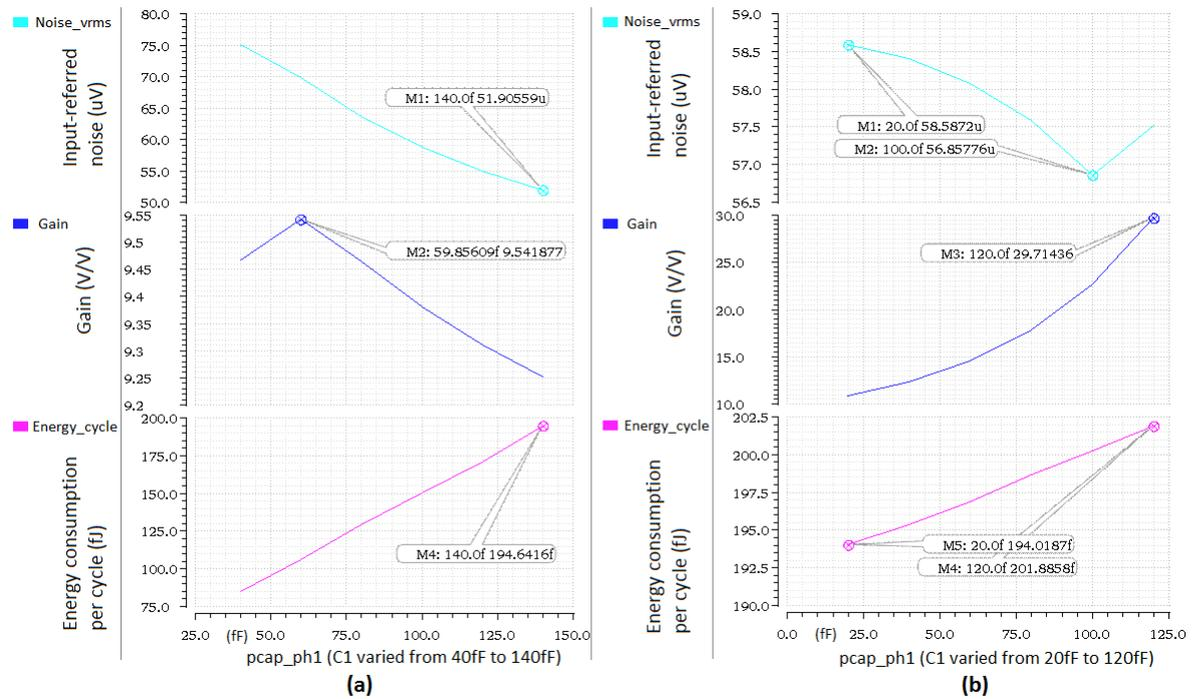
FIGURE 4.7: (a) The input-referred noise, gain and energy consumption of the single-stage integrator. Capacitor ( $C_1$ ) is varied from 40 fF to 140 fF (b) The input-referred noise, gain and energy consumption of cascoded integrator. Ratio between  $C_1$  and  $C_2$  is varied while keeping ( $C_1 + C_2$ ) constant (equal to 140 fF)
