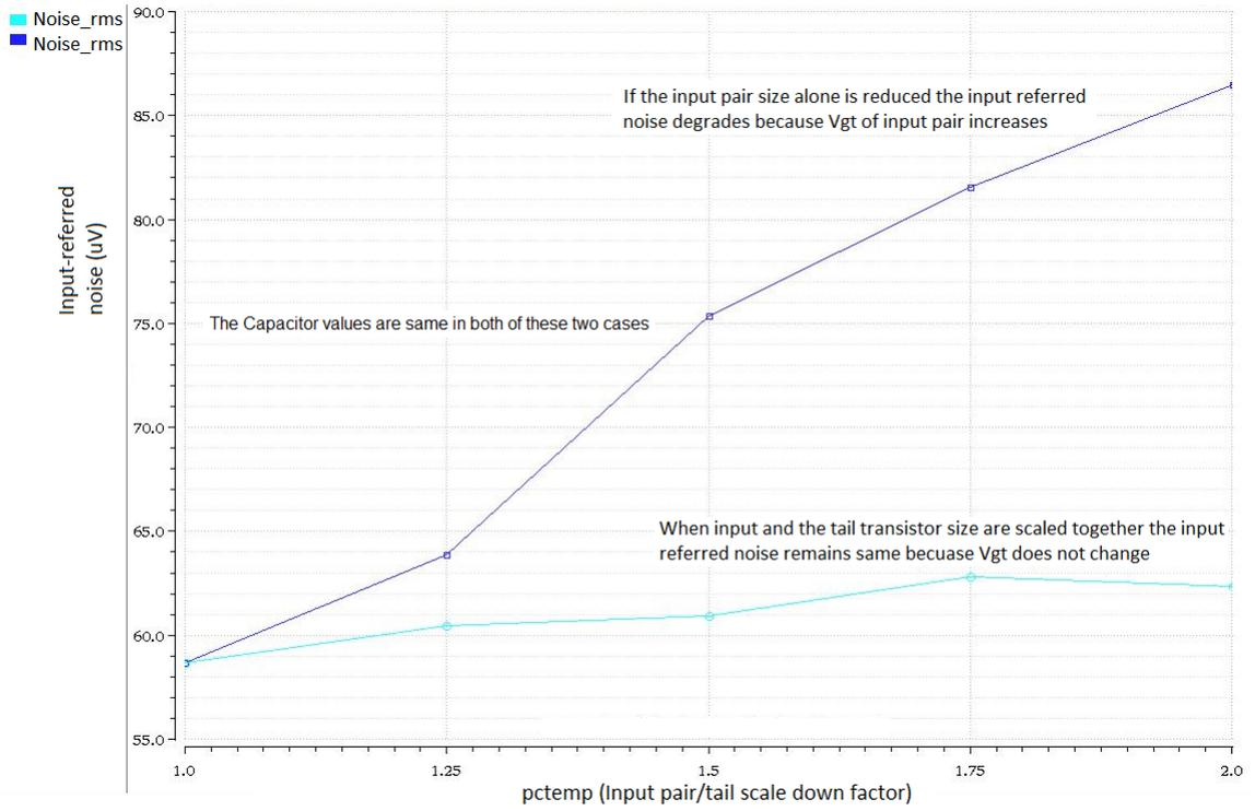
FIGURE 5.9: Input-referred noise versus the aspect ratio ( $\frac{W}{L}$ ) scale down factor (pctemp) for input pair and tail transistor.
