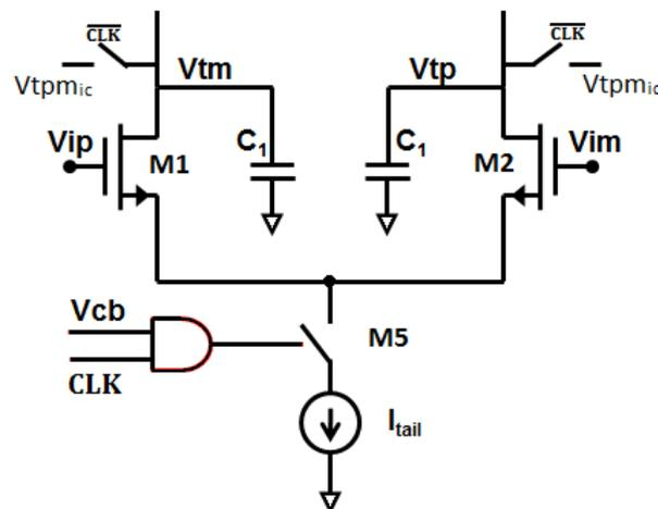
FIGURE 6.3: Tail current source for integration time configuration
