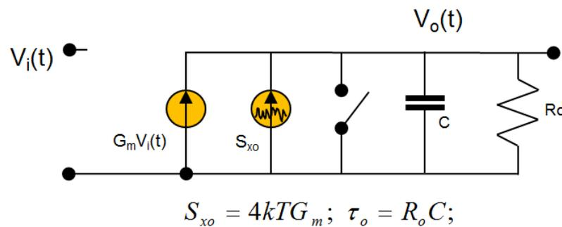
FIGURE 3.2: Transconductance amplifier model ( $t \leq 0$  switch is closed;  $t > 0$  switch is open)
