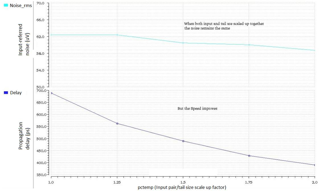
FIGURE 5.10: Input-referred noise and time delay versus the aspect ratio ( $\frac{W}{L}$ ) scale up factor (pctemp) for input pair and tail transistor.
