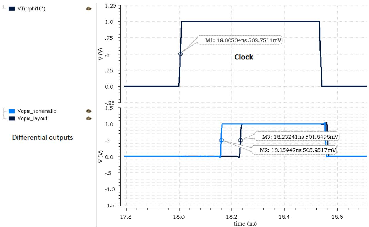
FIGURE B.6: PLPDC-2 : Differential output voltage of schematic and post layout simulations
