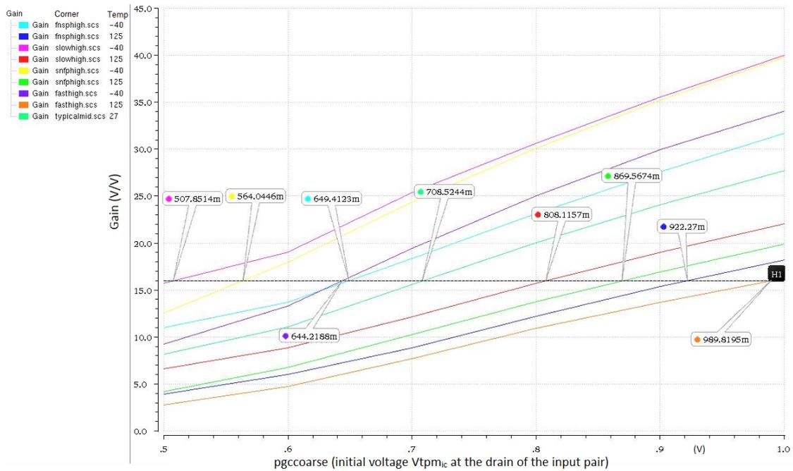
FIGURE 6.2: Gain versus  $V_{tpmic}$  (pgccoarse in the picture) across process and temperature corner
