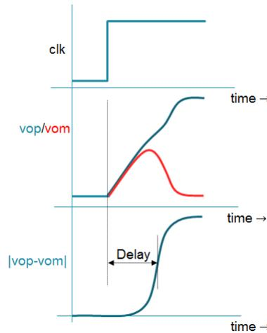
FIGURE 5.5: Comparator delay measurement
