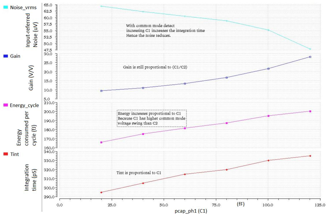
FIGURE 4.14: The input-referred noise, gain, energy and integration time as a function of  $C_1$  ( $pcap\_ph1$ ), where  $C_1 + C_2 = \text{constant}$ .
