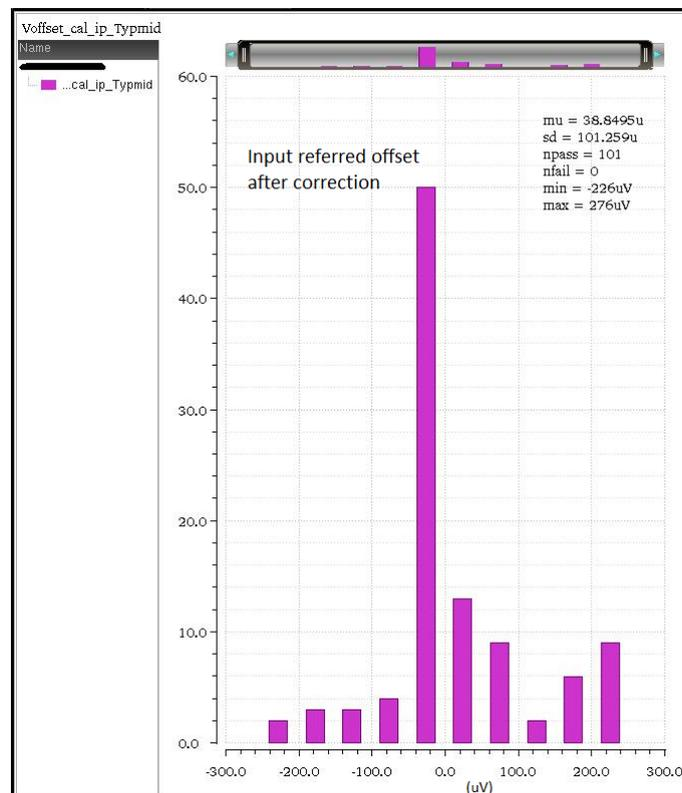
FIGURE A.11: Comparator-1 : Input referred offset after correction
