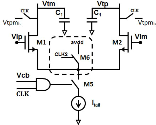
FIGURE 6.5: Switch for flicker noise reduction
