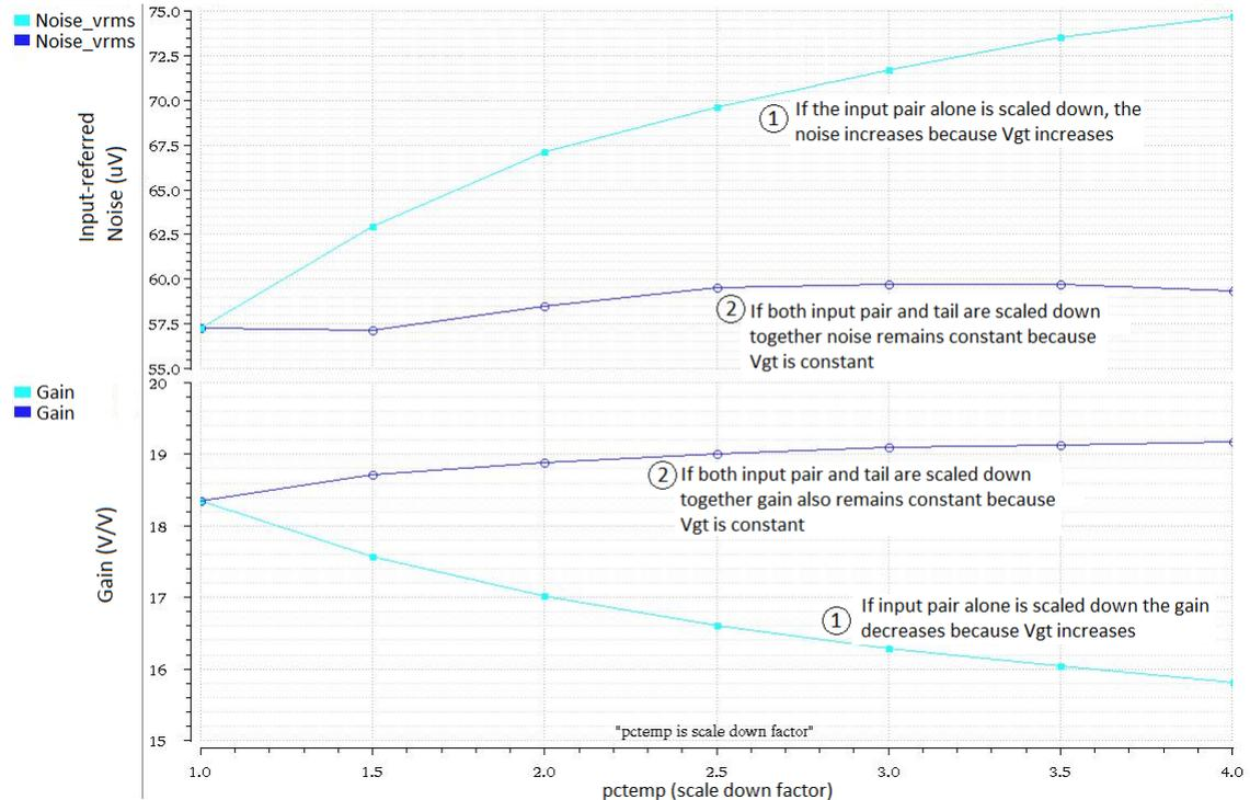
FIGURE 4.15: Input-referred noise and gain versus the aspect ratio ( $\frac{W}{L}$ ) scale down factor (pctemp) for input pair and tail transistor.
