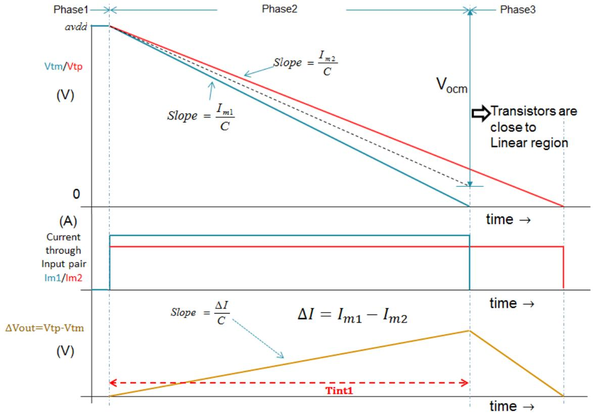
FIGURE 4.2: Graphical explanation of single-stage integrator functionality
