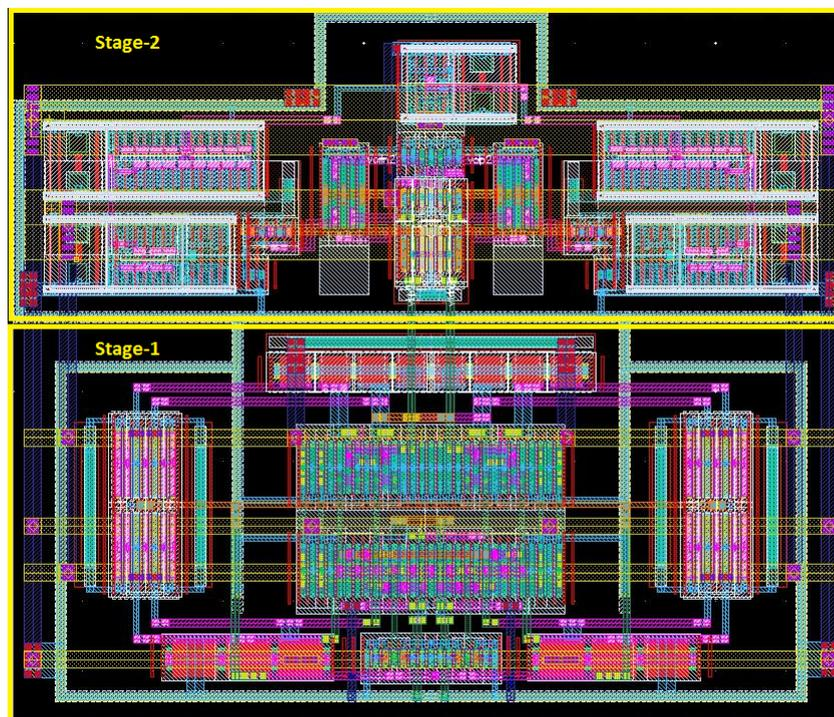
FIGURE B.3: PLPDC-2: Layout, and the size (width,height) of this module is  $(12\mu\text{m},11\mu\text{m})$
