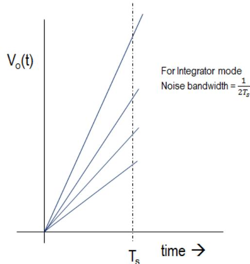
FIGURE 3.4: Step response of transconductance amplifier in the integrator mode versus time for different  $\frac{G_m}{C}$  values
