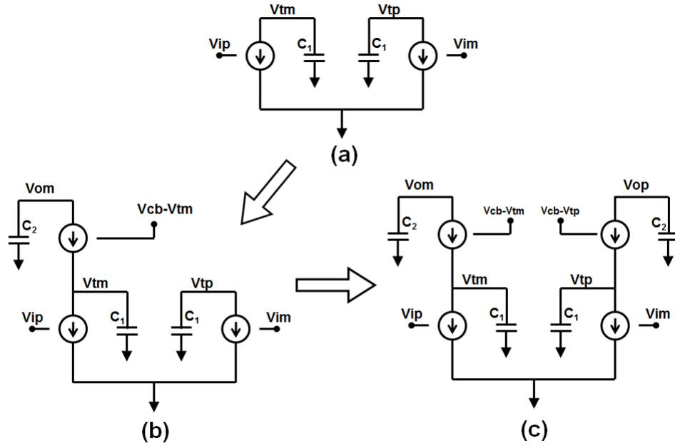
FIGURE 4.4: Small signal models of Figure 4.3 (a) for phase-2 (b) for phase-3 (c) for phase-4
