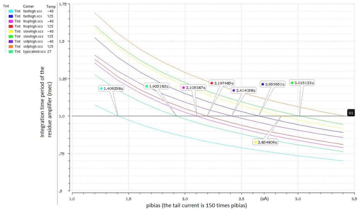
FIGURE 6.4: Integration time Vs tail current (150 times pibias)
