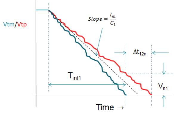
FIGURE 4.6: Calculation of the period  $\Delta t_{12n}$  due to the noise
