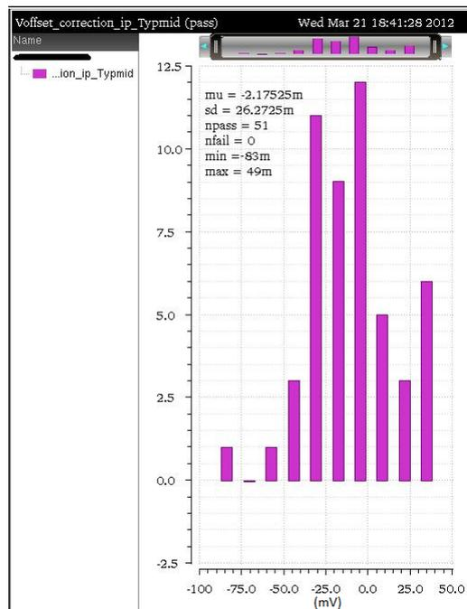
FIGURE A.15: Comparator-2 : voltage at gate of parallel input pair to cancel offset
