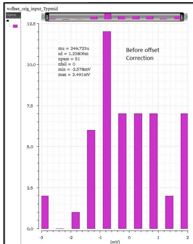
FIGURE A.4: CIDRA : Input referred offset before correction
