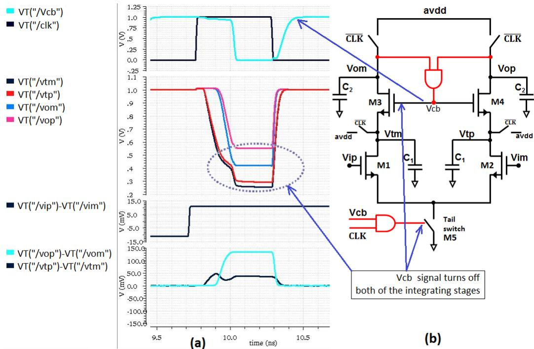
FIGURE 4.12: The transient simulation of CIDRA (a) One transient cycle (b) the CIDRA circuit (see Table 4.1 for parameters)
