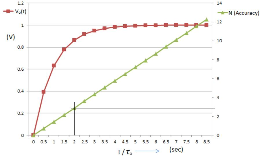
FIGURE C.2: Step response of the transconductance amplifier and accuracy (bits) versus normalized settling time
