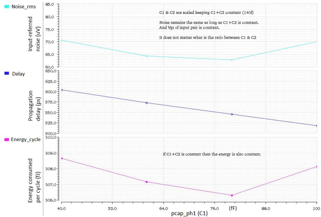
FIGURE 5.8: Input-referred noise, gain, energy and time delay as a function of  $C1$  ( $pcap\_ph1$ ), where  $C1+C2=\text{constant}$ .
