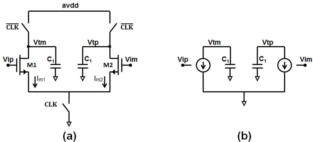
FIGURE 4.1: (a) Single-stage integrator (b) Equivalent small signal model of single-stage integrator
