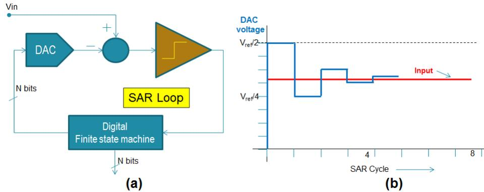
FIGURE 2.1: (a)SAR loop (b)5 cycles of SAR Loop with binary DAC
