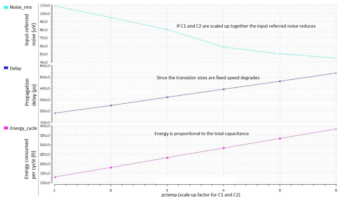
FIGURE 5.7: The input-referred noise, energy and delay as function of  $C_1$  and  $C_2$ . The variable pctemp is the scale up factor for  $C_1$  and  $C_2$ .
