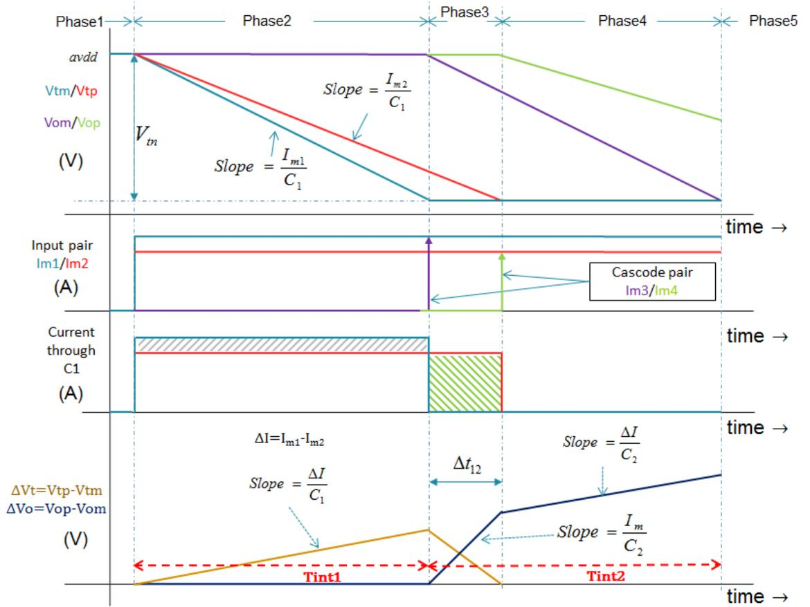
FIGURE 4.5: Graphical explanation of cascoded integrator functionality ( $C_1=C_2=C$ )
