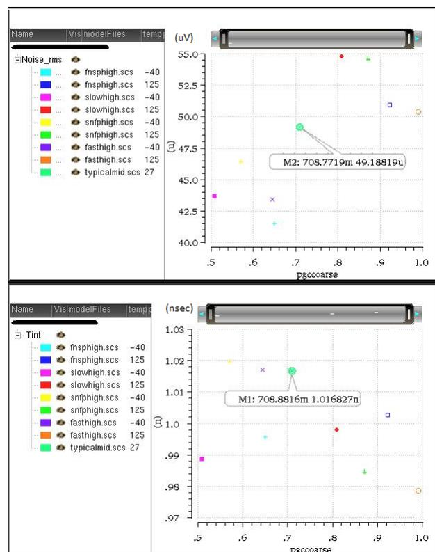
FIGURE A.2: CIDRA : Temperature and Corner simulations results of Noise(input referred) and Integration time
