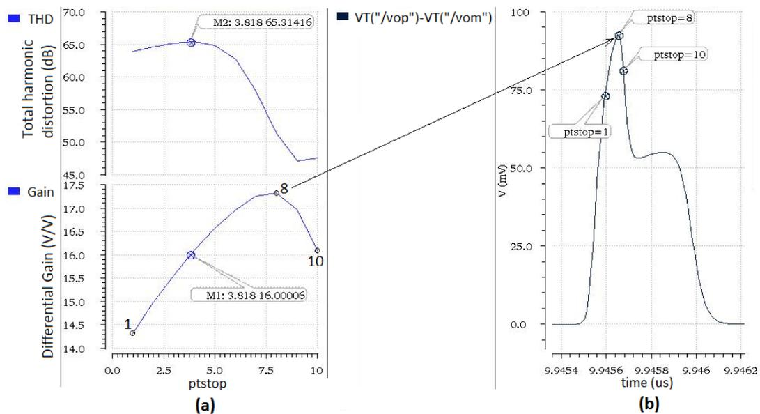
FIGURE 4.8: Simulation of linearity of the cascoded integrator with two-tone (50 MHz and 51 MHz) input with 11 mV pk-pk (see Table 4.1 for other parameters) (a) THD and gain versus sampling instance (ptstop) (b) Differential outputs versus time
