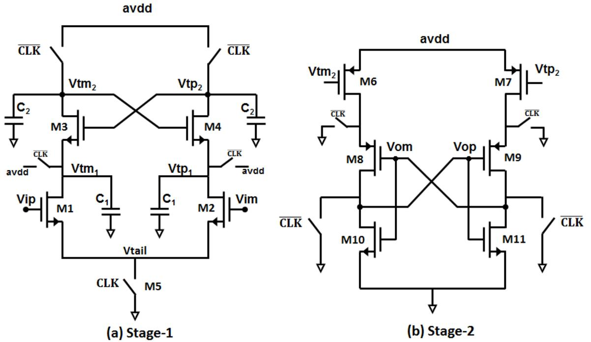
FIGURE 5.3: Pseudo-latch preamp dynamic comparator
