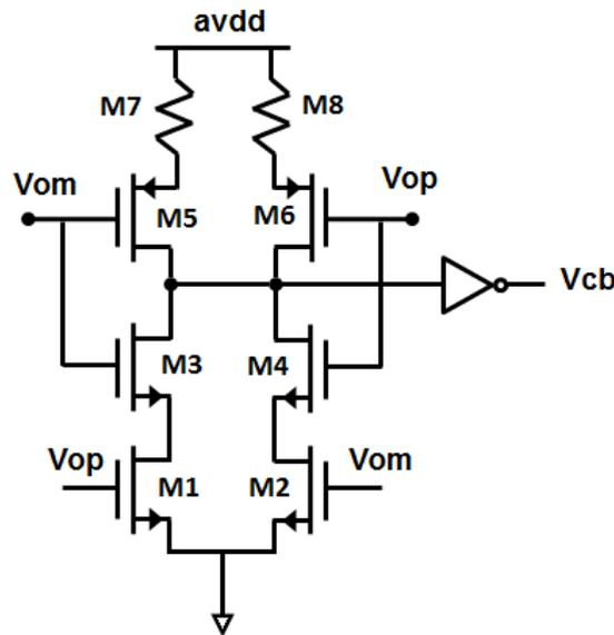
FIGURE 4.13: A symmetric common-mode detect circuit with source degeneration
