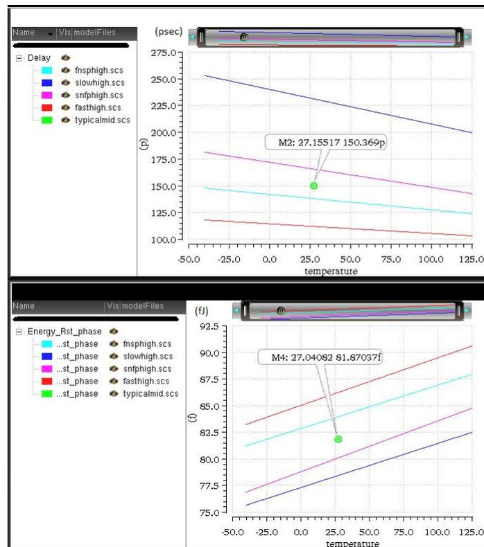
FIGURE A.7: Comparator-1 : Temperature and Corner simulations results of Delay) and Energy/cycle in the reset phase
