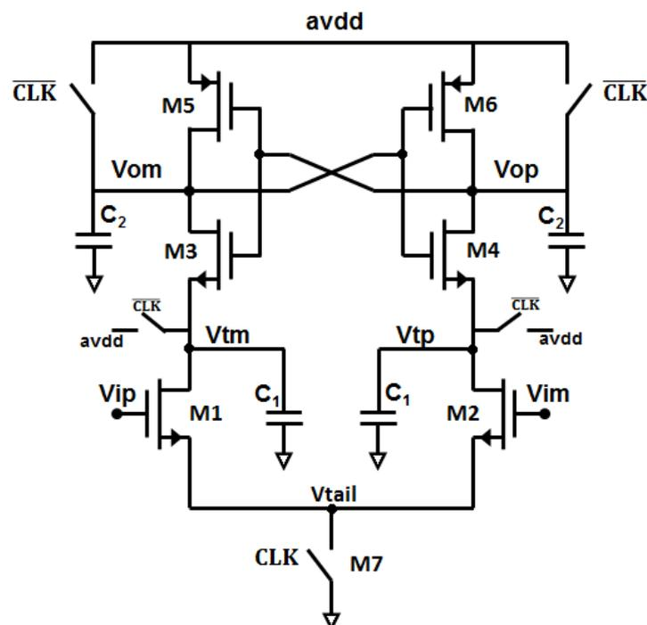
FIGURE 5.1: Sense amplifier based comparator
