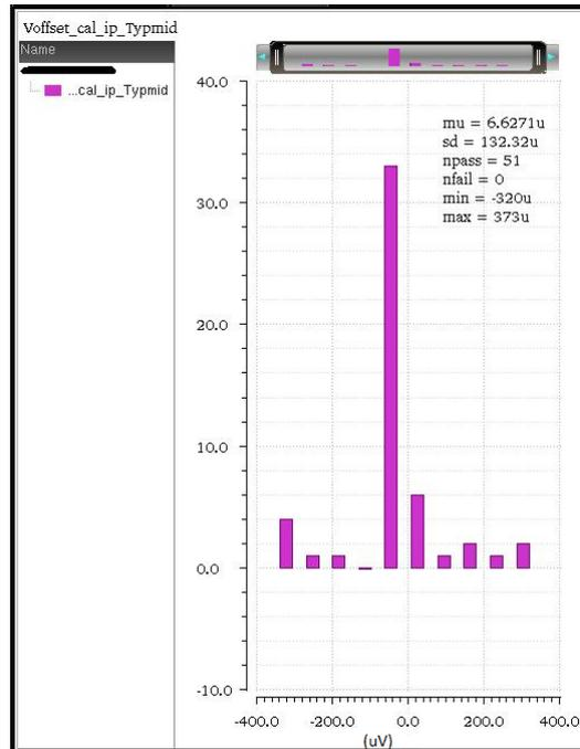
FIGURE A.14: Comparator-2 : Input referred offset after correction
