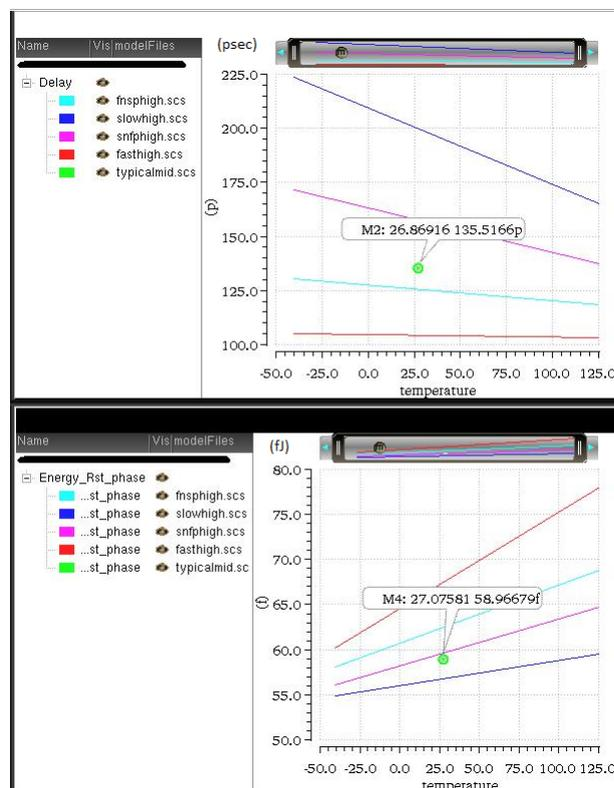
FIGURE A.9: Comparator-2 : Temperature and Corner simulations results of Delay) and Energy/cycle in the reset phase
