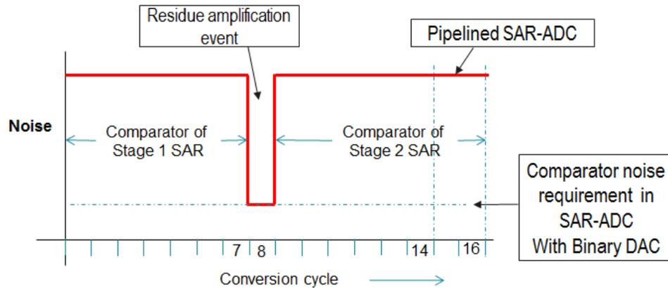
FIGURE 2.3: Comparator/residue amplifier noise requirement for SAR-ADC and pipelined SAR-ADC
