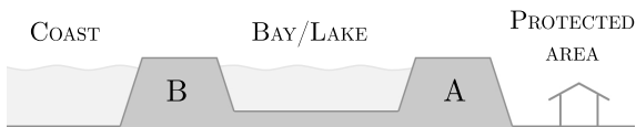
Figure 2.1: A hypothetical cross section of a coastal flood defence system with a front defence (B) and rear defence (A). In case the front defence breaches, the loads on the rear defence will increase.
