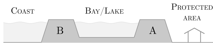
Figure 3.1: Simplified cross section of a front defence (B) and rear defence (A).
