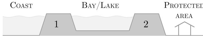
Figure 4.20: A coastal system with two lines of defence. This figure is an adaption from an illustration found in [26].
