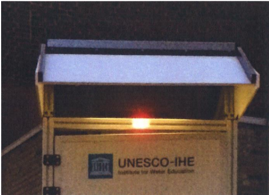
Figure 3-13 Occupancy light activated in eSOS Smart Toilet immediately after the user steps in (Photo: J. Čurko)
