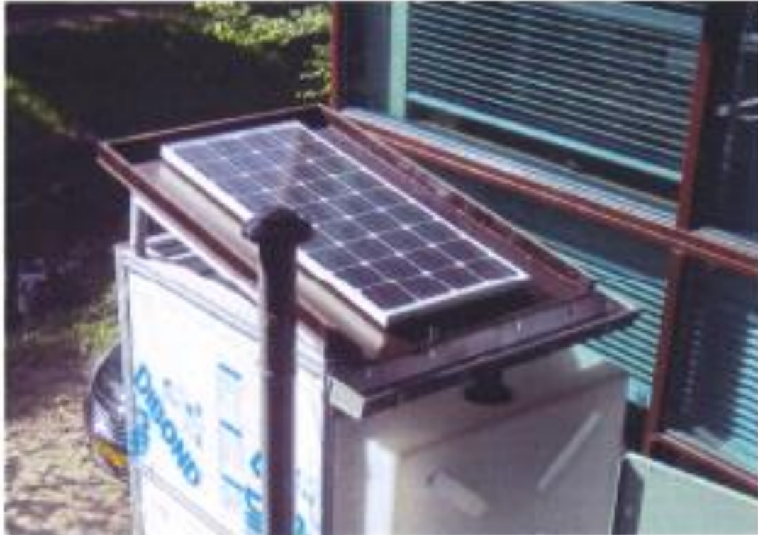
Figure 3-7 Solar panel mounted at the top of the eSOS toilet at optimal angle for maximum efficiency (Photo: D. Brdjanovic)
