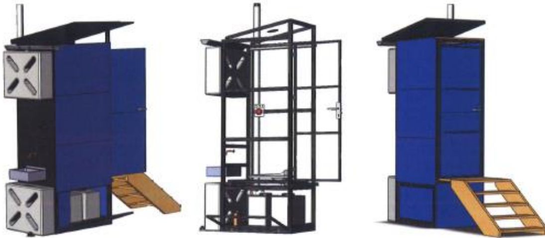
Figure 3-2 The conceptual design of the experimental eSOS Smart Toilet (Images: Flex/design)
