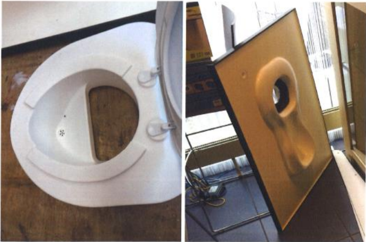
Figure 3-5 Interchangeable user interface used in the experimental eSOS Smart Toilet (Photos: D. Brdjanovic)
