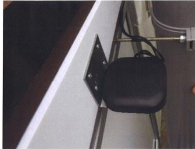
Figure 3-10 GSM antenna at the top of the experimental eSOS Smart Toilet (Photo: D. Brdjanovic)
