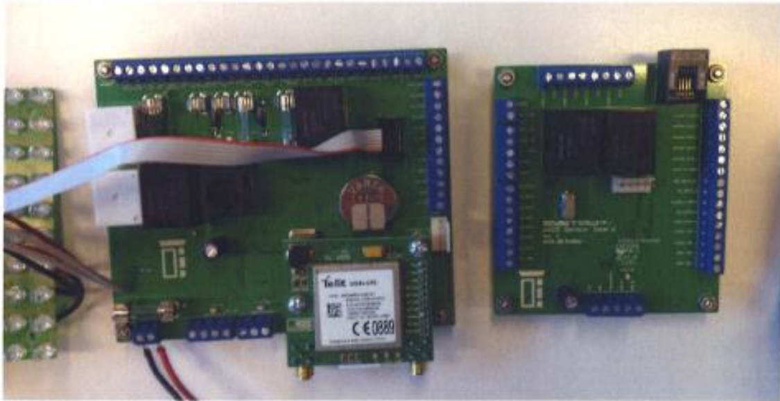
Figure 3-9 Tailor-made electronic components of eSOS CPU (Photo: A. Muratbegovic)
