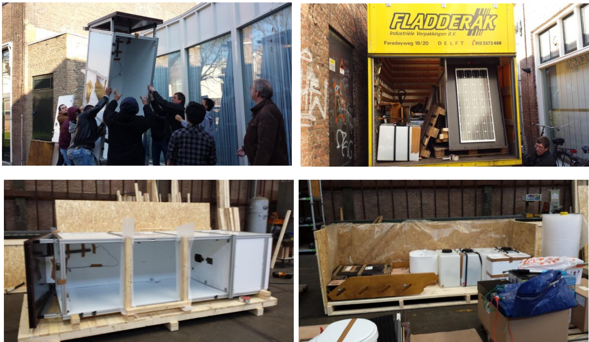
Figure 3-35 Shipment Process in Delft – Top: Dissembled toilet structures were being loaded to the truck to further be packed by packing company; Bottom: Packing process by packing company into 2 shipment crates (Photos: F. Zakaria)
