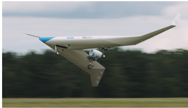
Figure 2.3: Flying-V scale model first test flight 1
