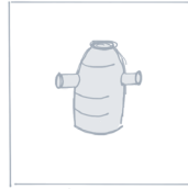
"Vortceptor": hydrodynamic separator (captures pollutants, sediment, oil)
