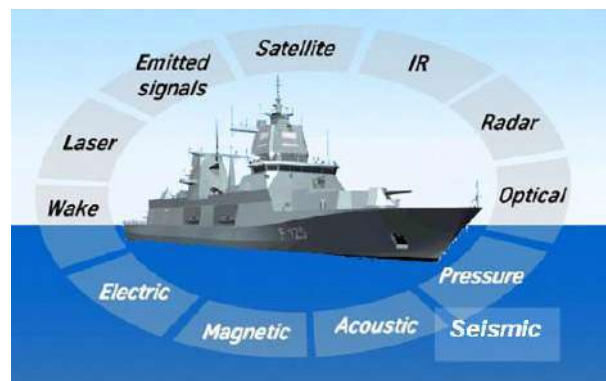
Figure 1.1: Overview signatures naval vessel [23]
