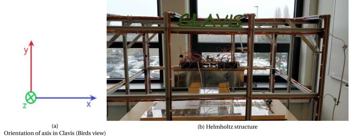
Figure 7.2: Helmholtz structure 'Clavis' and axis orientation
