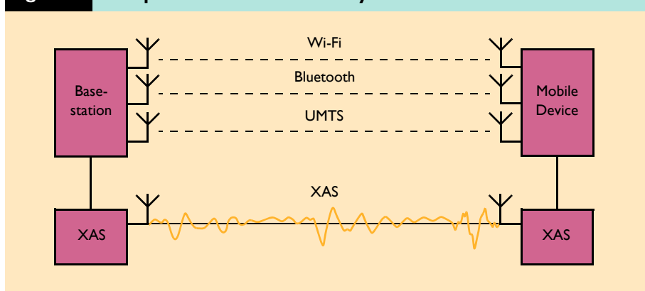
Figure 2 Set-up of the advertisement system XAS
