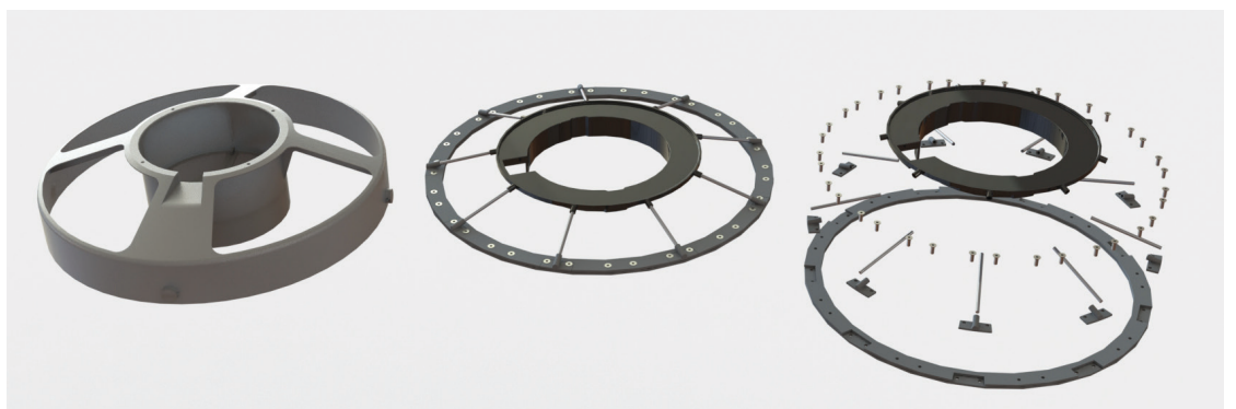
Figure 31. Comparison between the first render of a 'unified' canopy and the M-Tego I prototype canopy assembled and in exploded view.
