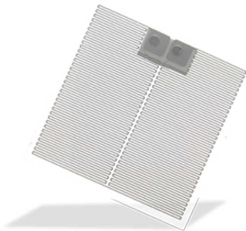
Figure 54. A polyester heating element. A great variety exists of plastic carriers with each their own properties. Polyester is cheap, flexible and durable.
