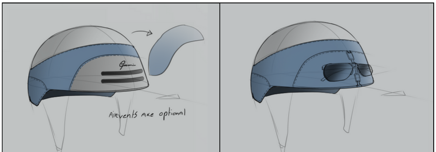
Figure 31. Fabriqu   helmet different configurations: open airvents and holding sunglasses
