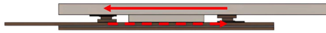
FIGURE 14. Hybrid power module with planar connection (for power loop) and wire bonding (for gate-loop) [76].
