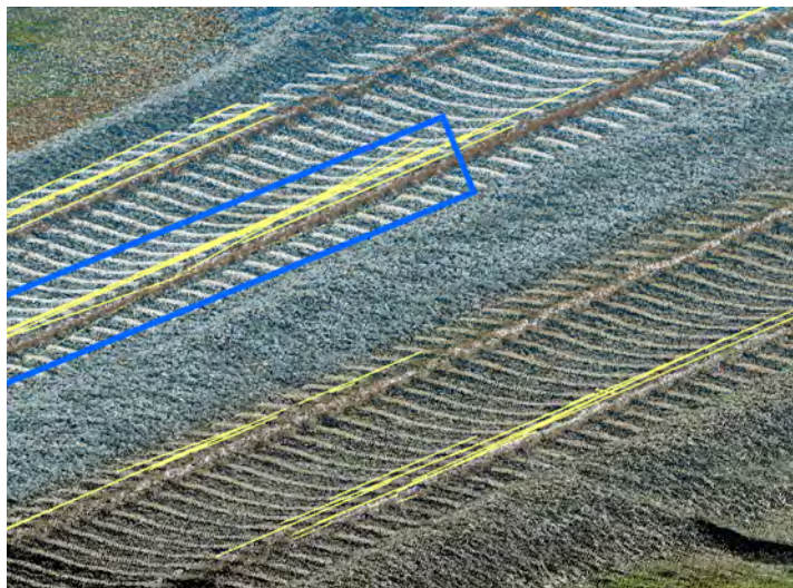
Figure 4.15: Best results for reconstruction found in the Stroe data-set. Reconstructed lines shown in yellow. Although most lines are in the general direction and location of actual rails, some lines have a vertical component which does not exist in reality (highlighted by the blue border).
