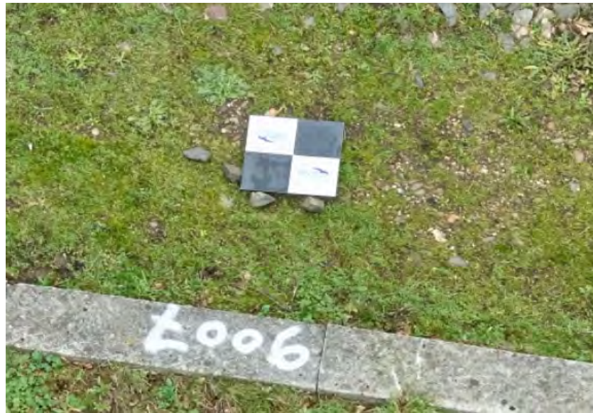
Figure 2.9: Ground control point example for Stroe dataset
