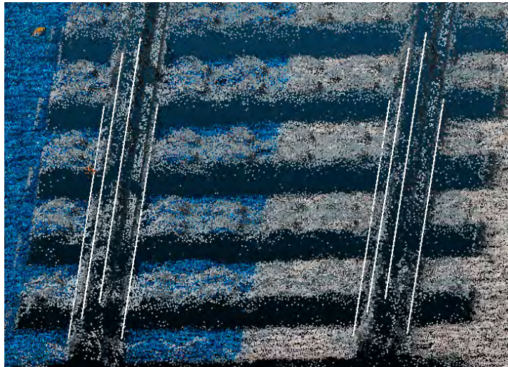
Figure 4.10: Reconstruction of manually matched Lego data. The white reconstructed lines resemble the rail from the photogrammetric point-cloud, two lines per rail show the top and two lines the bottom of the rail.
