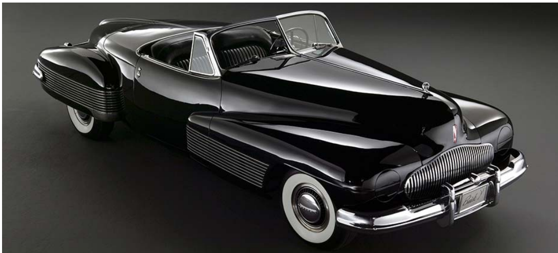
Figure 3 Prototype of the Buick Y-Job. The Y-job included novel characteristics such as “hidden headlamps, electrically operated windows, flush door handles and a power-operated convertible top” (Dream Car 1938, 2012). Image by http://www.buick.com/experience/heritage.html
