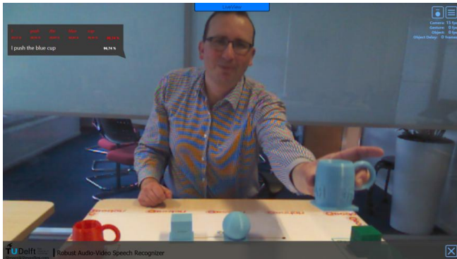
Fig 4-3 An active ASR, showing the result in a speech bubble
