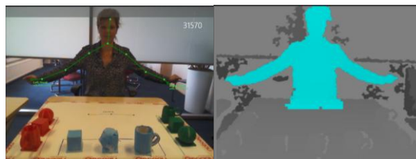
Figure 3-4 Sensors in the Kinect V1 Figure 3-5 Raw data (RGB+skeleton left, Depth right)
