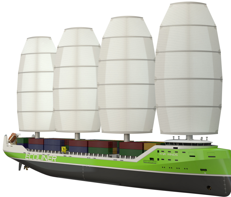
Figure 2-1: Render of the Ecoliner , design by Dykstra Naval Architects (Nikkels, 2013)
